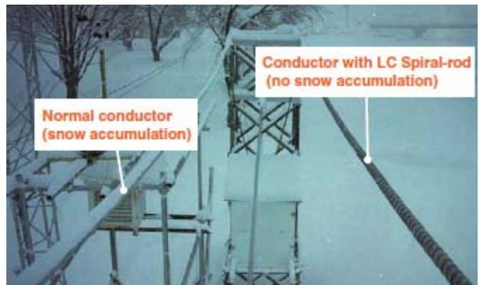
Fig. 6. Example of evaluation test results at a snow test site.
