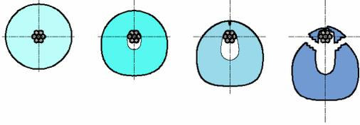
Fig. 1 Process of snow creep (re-draw from [2])
