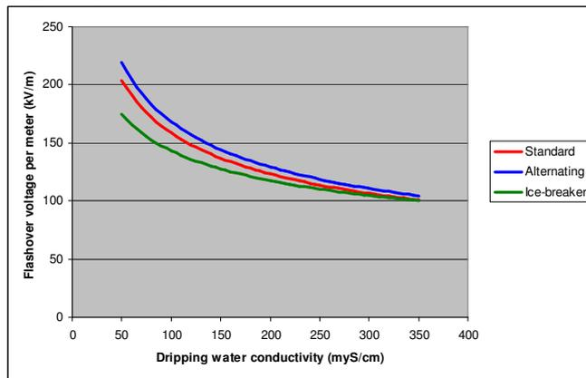
Figure 11 Pollution performance curves derived from freezing rain tests (5 hours ice accretion time).
