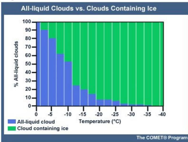
Fig. 1. Percentage of cloud phase (liquid/mixed) as a function of temperature [1].
