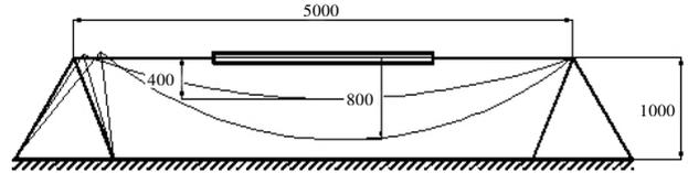
Fig. 3. Geometry of experimental cable with different sags
