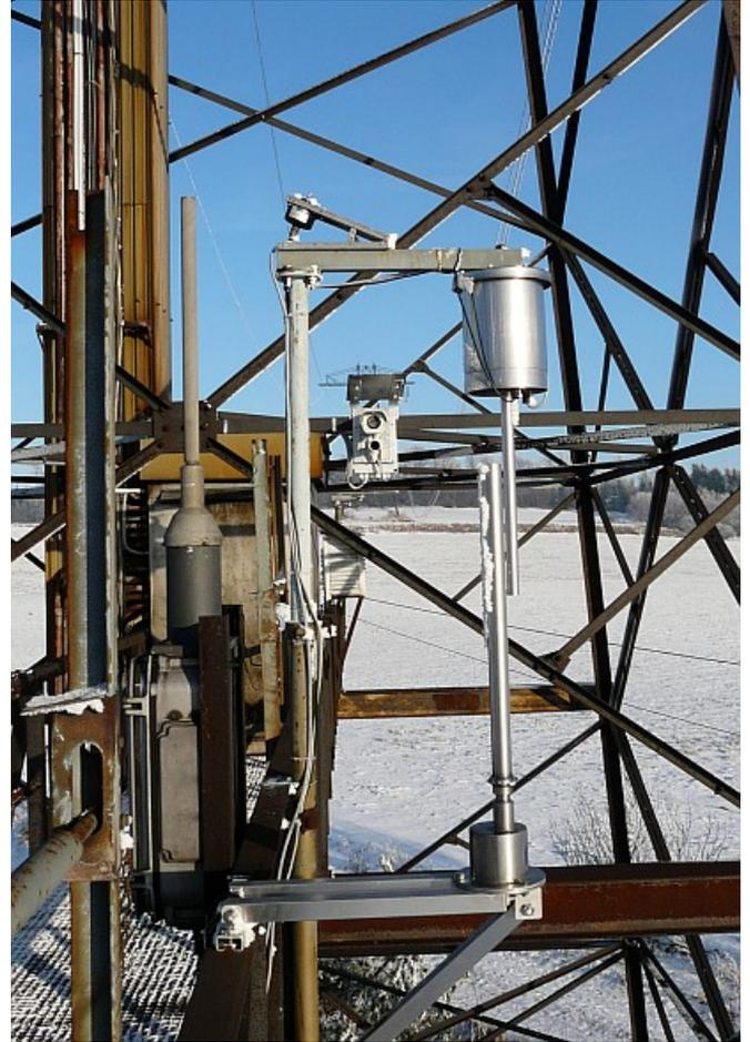
Fig. 8 Video coverage of IceMonitor, Goodrich, PMS and vertical rod
