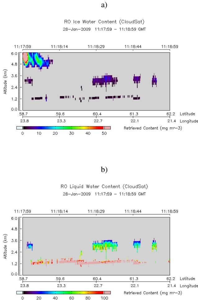
Fig. 5. a) Ice water and b) liquid water content measured by CloudSat [6].
