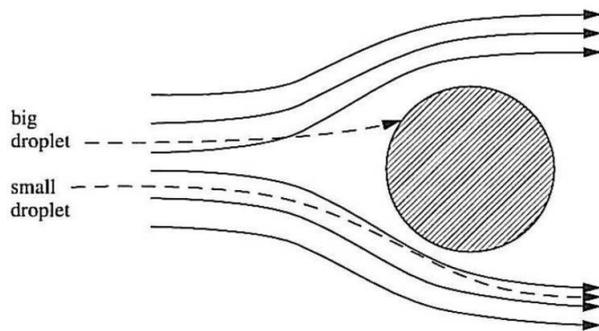
Fig. 1. Air streams and droplet trajectories around a cylindrical object (sketch taken from Makkonen, 2000).
