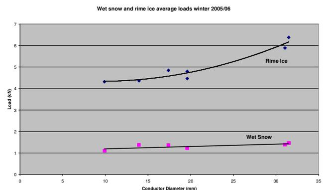
Fig. 4.4 Averaged rime ice and wet snow loads against conductor diameter from Deadwater Fell tests
