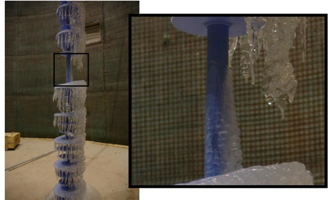
Figure 7 Ice-breaker profile with close to complete bridging of the long gap.
