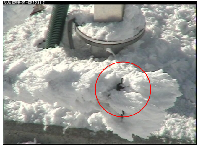
Picture 5: Goodrich Ice detector encapsulated in rime ice.
