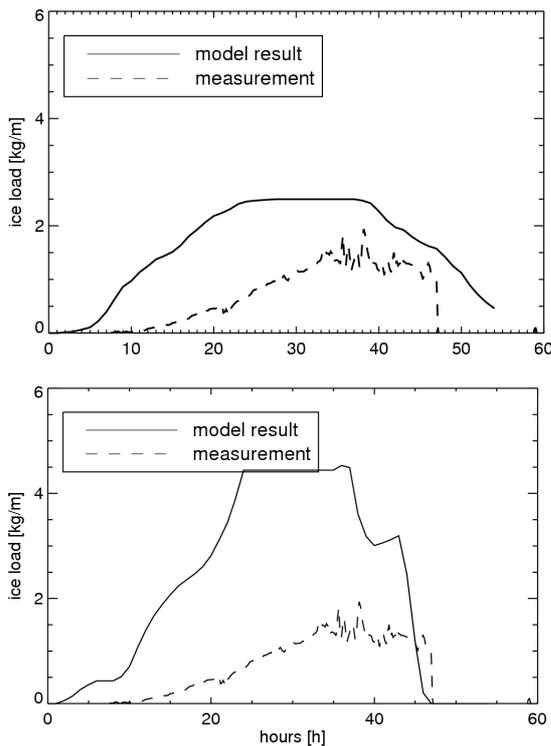
Fig. 4. Time series of simulated ice load at the position of Schwyberg for a simulation starting on 13.11..2008, 00 UTC using WRF (upper panel) and COSMO results (lower panel) as input. Measurements are shown as dashed line, the model results as continuous line.
