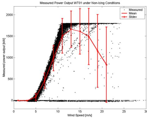
Fig. 7: Power output wt01 under non-icing conditions.
