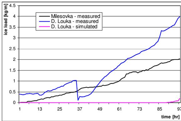
Fig. 5. Measured and simulated ice load of icing event in Dec2007 at Milešovka Mt. and Dlouhá Louka
