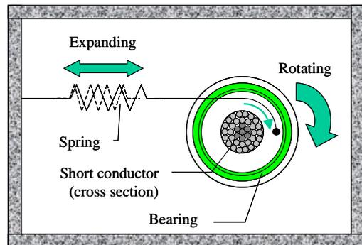
Fig. 7. Conceptual sketch of the apparatus that installs torsional rigidity
