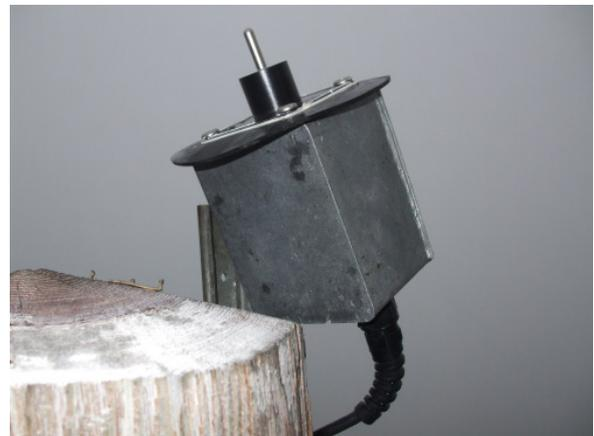
Fig. 3.3 The Rosemount mounted on one of the wood pole supports of the platform at Deadwater Fell.
