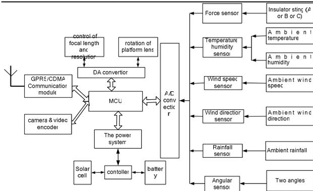
Fig.2 The block principle of online monitoring unit
