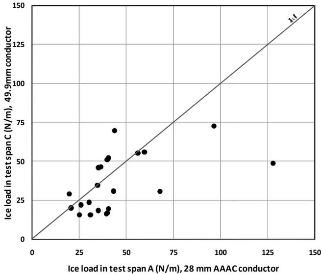
Fig. 20. Comparison between 28 mm AAAC conductor in test span A and 49.9 AACSR conductor in test span C.
