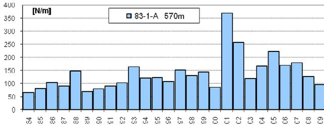
Fig. 9. Annual maximum ice load in test span A, incl. conductor weight
