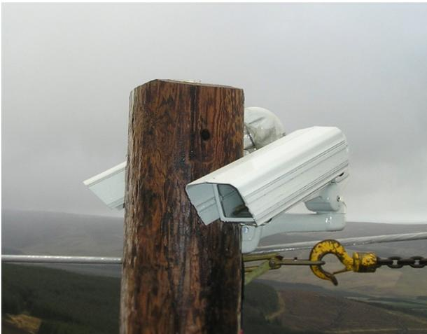
Fig. 3.1 Heated video cameras used for each conductor
