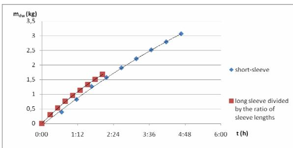
Fig. 12. Effects of sleeve length on the mass of dripping water
