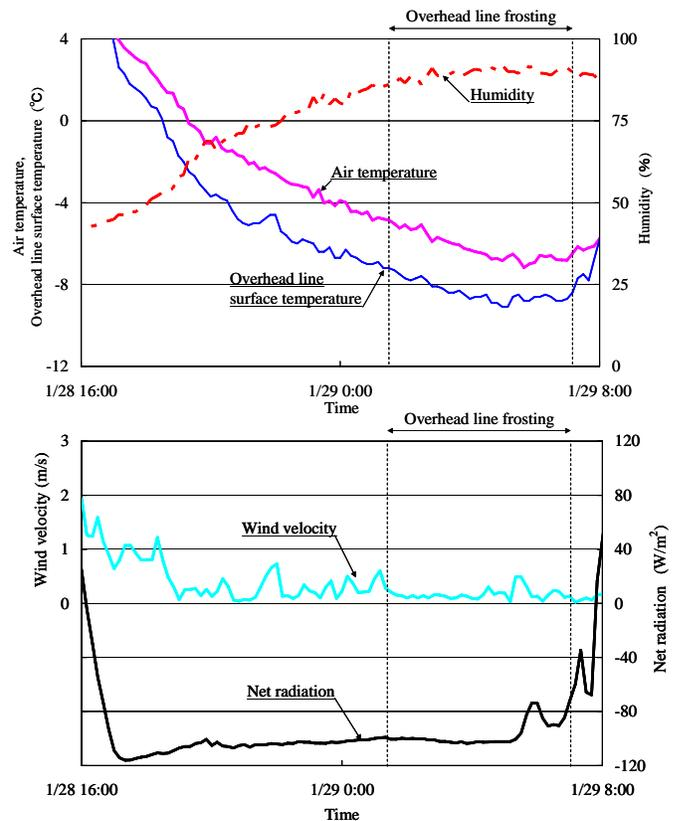
Fig. 4. Typical weather condition of overhead line frosting outbreak day
