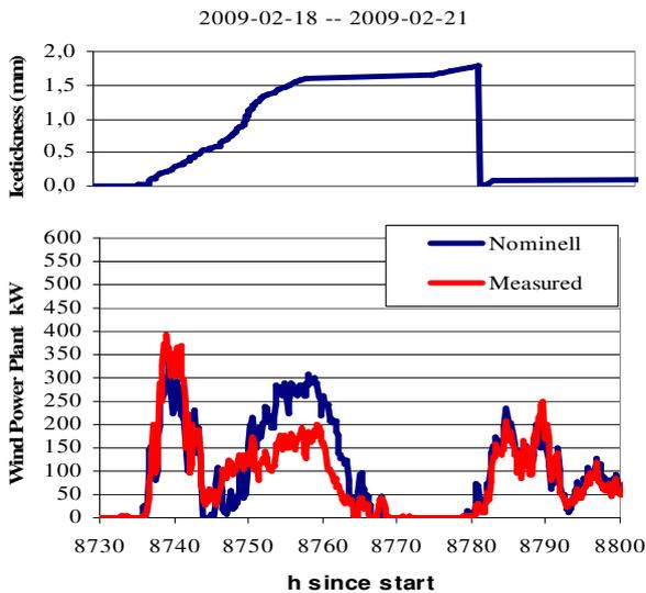
Fig 3 Härnösand Light icing on a wind power plant
