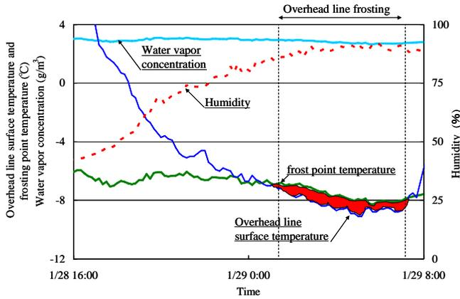
Fig. 9. Time change of overhead line surface temperature, frost point temperature, humidity, water vapor concentration. Frost point temperature and water vapor concentration are touched up on fig. 4.
