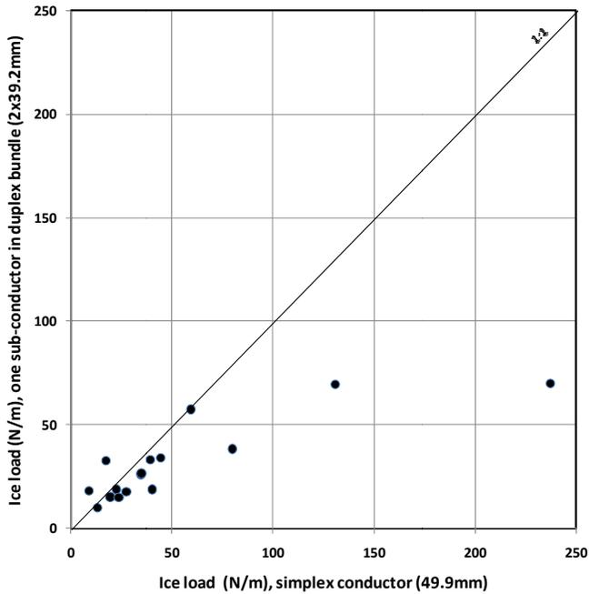
Fig. 13. Comparison of ice load on simplex conductor (49.9 mm) and one sub-conductor in duplex conductor (2x39.2 mm). Measurements are made in 400 kV OHTLs (FL3 and FL4).
