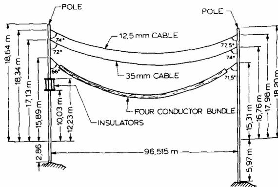
Fig. 4. Mt. Valin Test Span [17]
