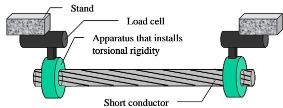
Fig. 6. Sketch of the test conductors
