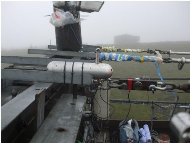
Fig. 3.2 Load cells and turnbuckles are installed on all conductors
