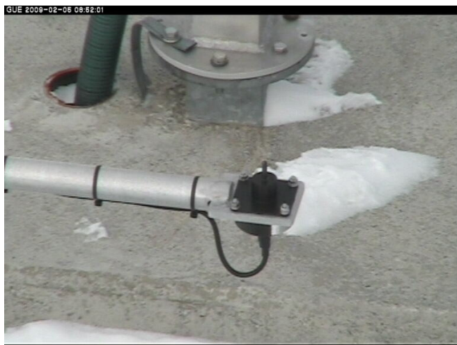
Picture 6: Goodrich Ice Detector on February 5 th .
