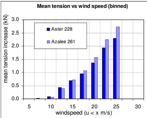
Fig. 4.5 Effect of wind only (no ice) on smooth (light blue) and stranded (dark blue) conductors of 19mm diameter
