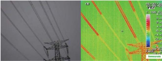
Fig. 7. Example of an infrared image (right-hand side) of the actual transmission line (left-hand side) with red parts corresponding to installed sections of LC-Spiral Rods.
