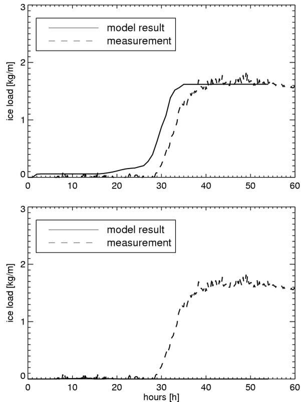
Fig. 5. Time series of simulated ice load at the position of Guetsch for a simulation starting on 22.11.2007, 00 UTC using WRF (upper panel) and COSMO results (lower panel) as input. Measurements are shown as dashed
