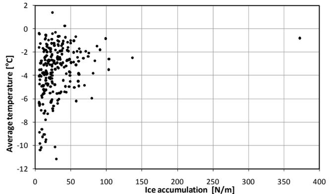
Fig. 7. Average temperature at the time of ice accumulation in test span A.
