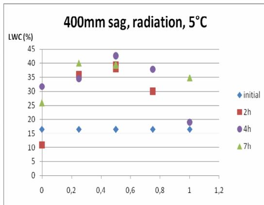
Fig. 6. Typical LWC distributions along the cable
