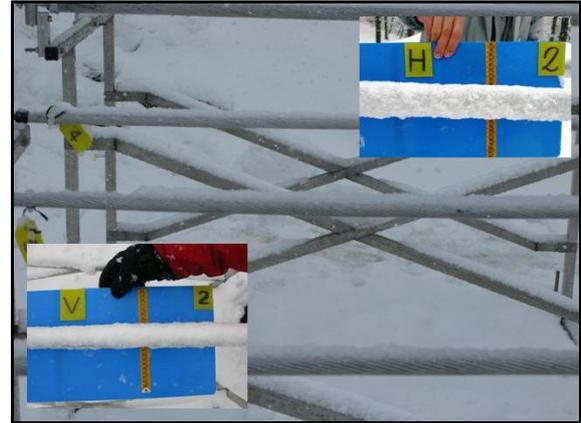
Figure 9: the ice diameter measurements. H is the shot on horizontal wire plane, V is on the vertical one.
