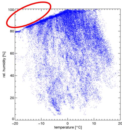
Fig. 3: Relative humidity measured according WMO/CIMO standards does not reach saturation anymore at temperatures below 0°C (red area).
