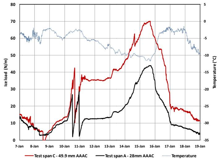
Fig. 22. Ice load in test span A with 28 mm AAAC conductor and test span C with 49.9 mm conductor during the period 7-19.Jan. 2008.
