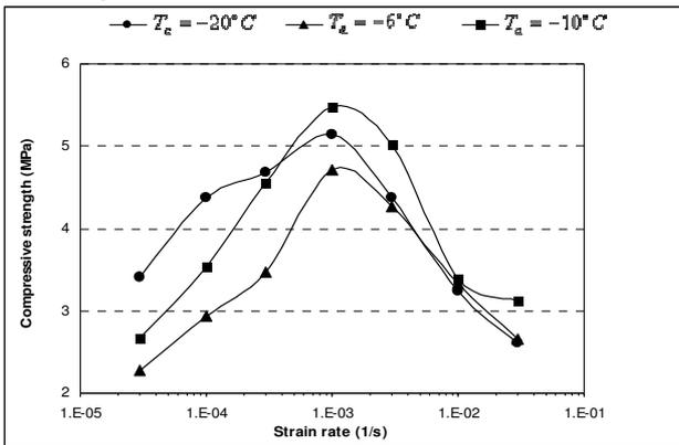
Fig. 3. Compressive strength of atmospheric ice accumulated at various temperatures and tested at their accumulation temperature.  $T_a$  = Accumulation temperature (Kermani *et al.*, 2007).
