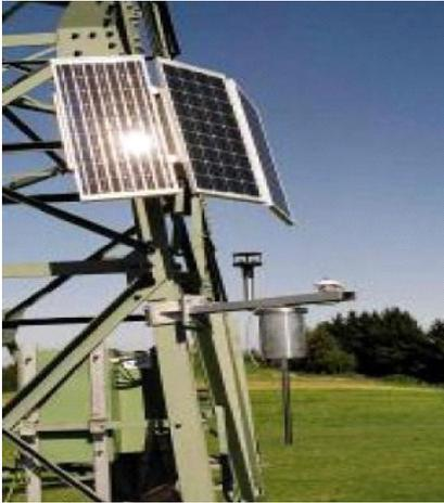
Fig. 2.2. The solar powered PMS icemeter (Courtesy EGU)
