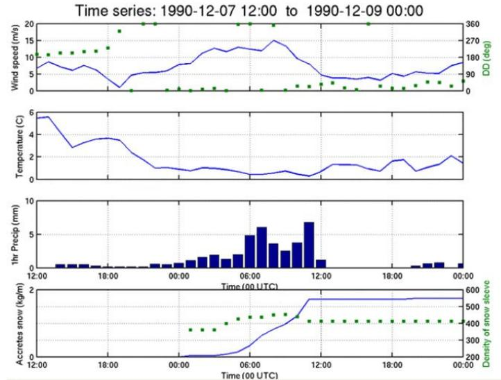
Fig. 8 The time period of wind speed, temperature, precipitation and accreted load of the storm
