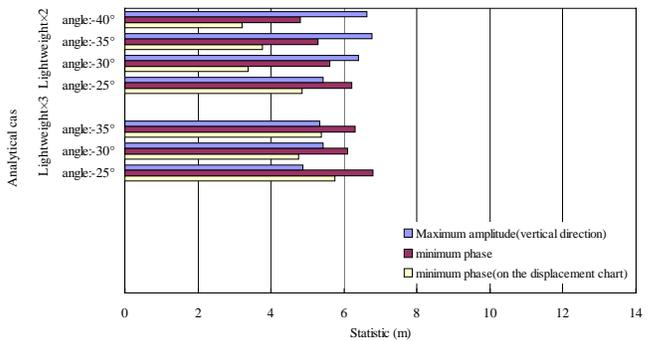
Fig. 7 (c) Comparison of statistics (Three equal spans: 400 m, Wind: 30 m/s, Leeward snow-accretion)
