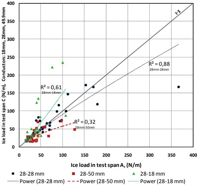
Fig. 24. Comparison of test span A (28 mm) to different diameter of conductors in test span C (18 mm, 28 mm, and 49.9 mm).
