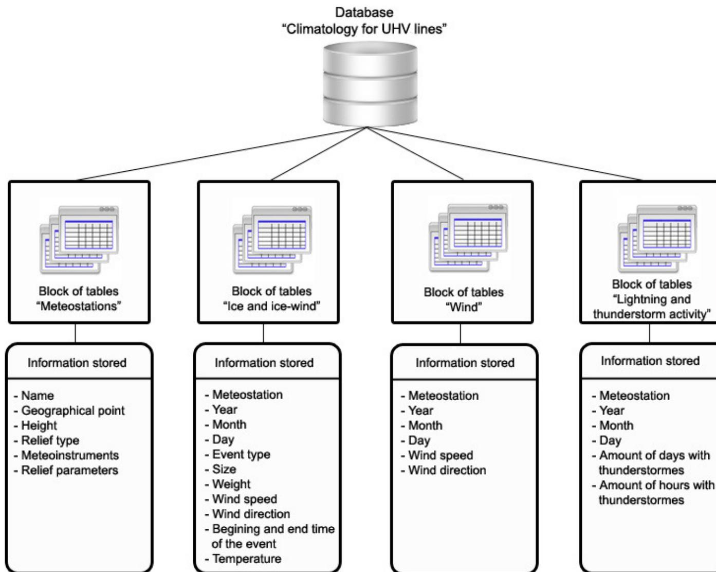
Figure 3: Logical scheme of the database for climate conditions
