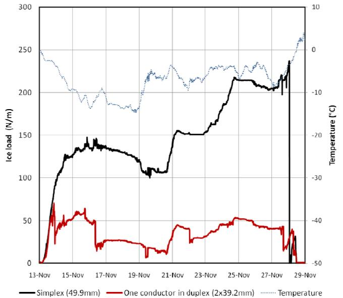
Fig. 14. Ice load on simplex conductor (49.9 mm) and one sub-conductor in a duplex conductor (2x39.2 mm) during the period 12-29 Nov.2006.
