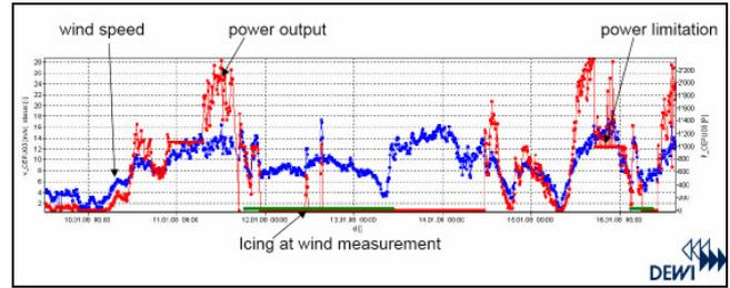
Fig. 4. French site: wt11, example for an icing period, wind speed, power output and icing status. The wind turbine stop persists longer than the ice at the parallel wind measurement.
