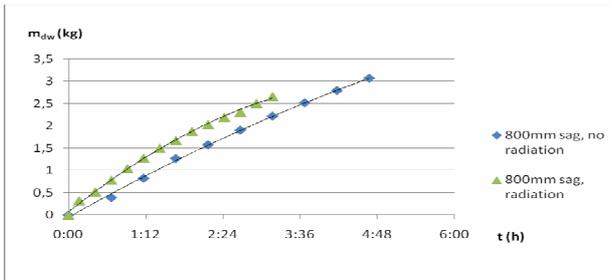
Fig. 10. Effect of radiation on mass of dripping water
