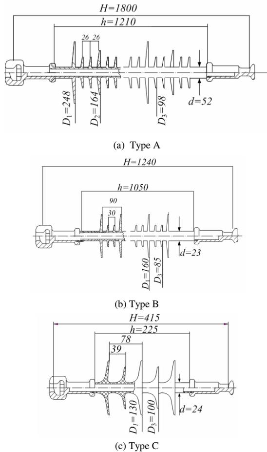
Fig.1 Sketch maps of the tested insulators
