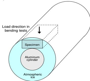
Fig. 1. Specimen position in accumulated atmospheric ice and load direction during test.
