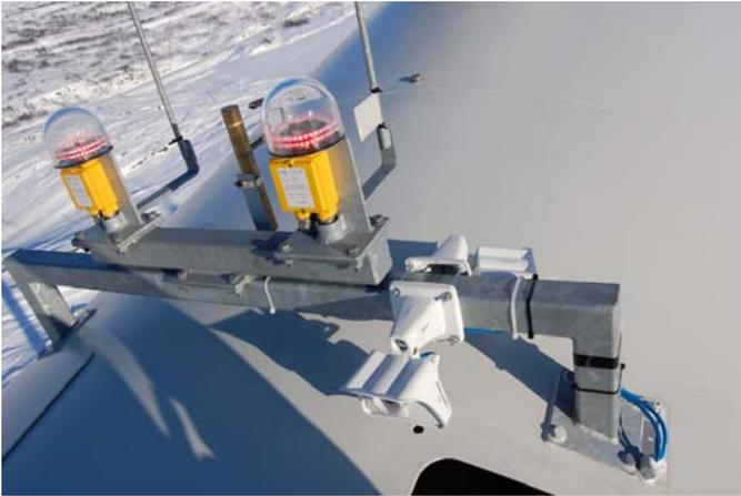
Figure 1: Web cameras installed on light boom.
