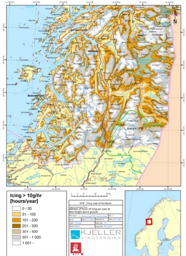
Fig. 3. Number of hours per year with ice accumulation
