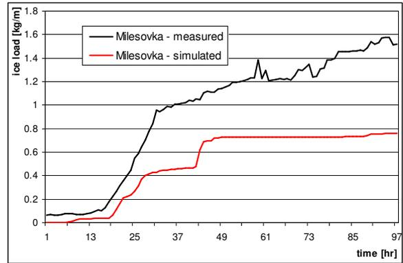
Fig. 4. Measured and simulated ice load of icing event in 2003/04 at Milešovka Mt.
