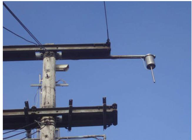
Fig. 2.1. The PMS icemeter installed at the upper crossarm of the southern H-pole on the Deadwater Fell test line.
