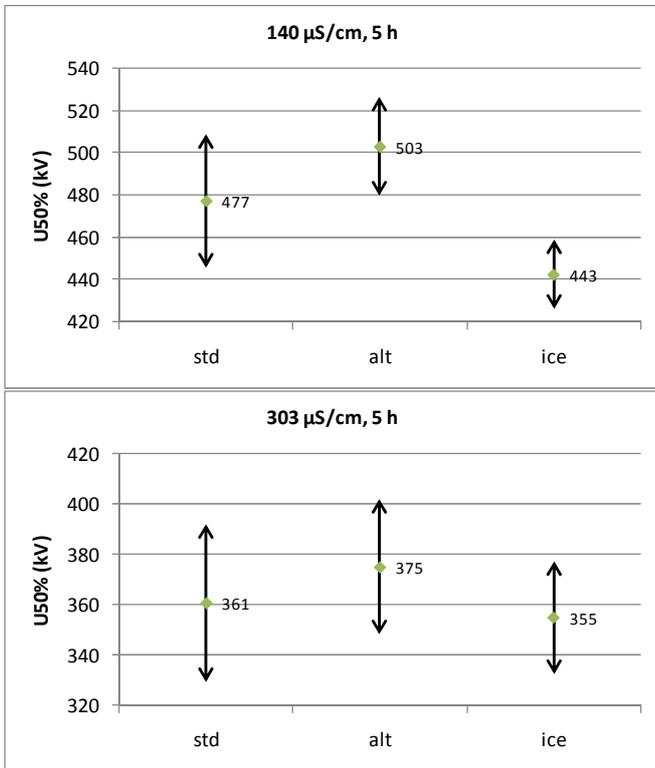
Figure 6  $U_{50\%}$ -values derived from tests with 5 h ice accretion. Error bars (arrows) correspond to one standard deviation.
