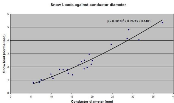
Fig. 4.1 Snow loads against conductor diameter for 28 conductors using data from the rotating rig. A polynomial fit is also shown.
