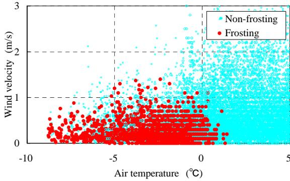
Fig. 6. Relationship between air temperature and wind velocity
