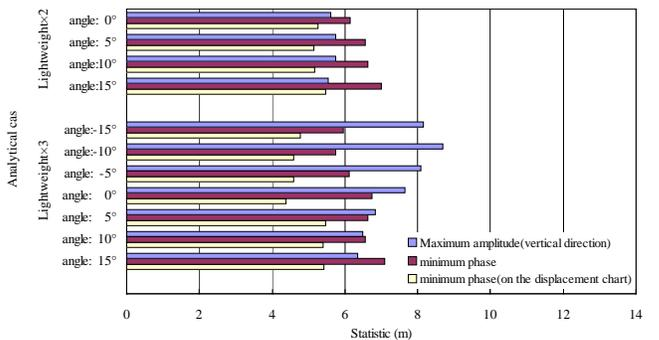
Fig. 7 (d) Comparison of statistics (Single spans: 400 m, Wind: 30 m/s, Leeward snow-accretion)
