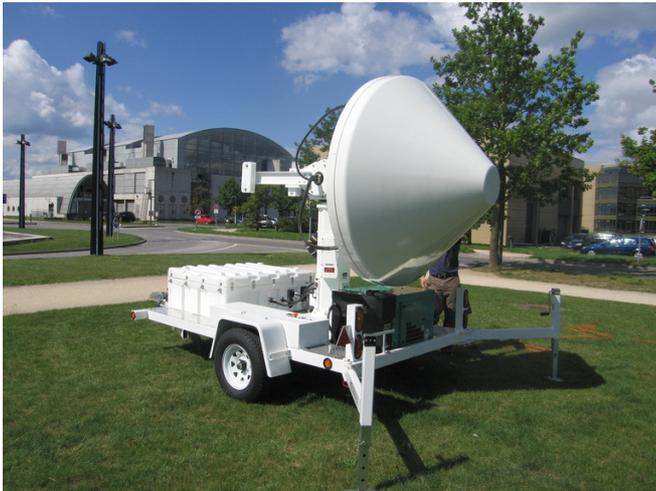
Fig. 2. The mobile X-band polarimetric radar system.
