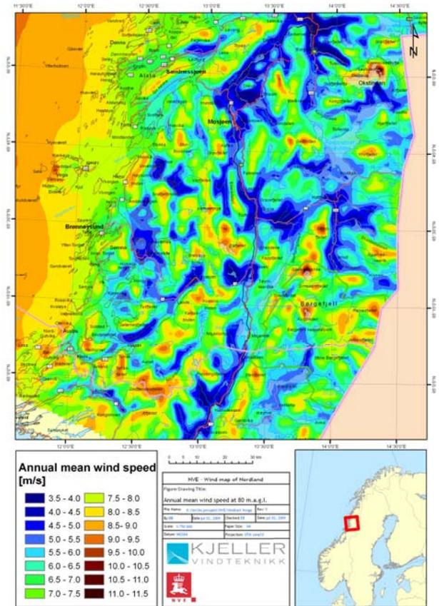
Fig. 2. Expected annual mean wind speed at 80m height.
