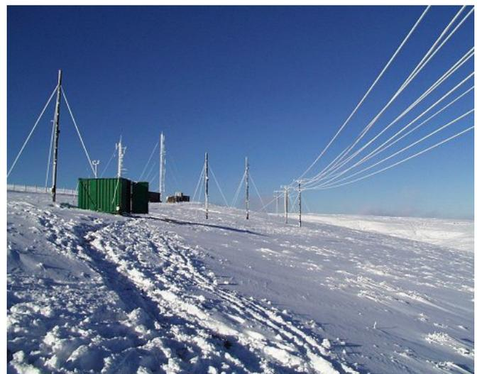
Fig. 2.2 The main test span and measurement huts plus poles for infra red lighting at the test site. In this picture intermediate single poles have been erected for testing small conductor sizes.
