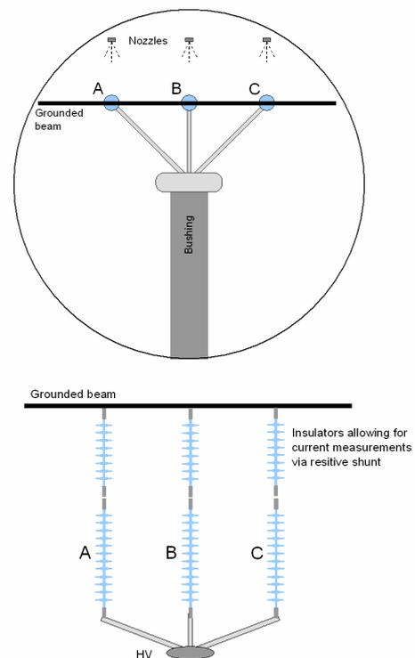
Figure 1 Schematic drawing showing insulators under test (A-C) hanging vertically in front of the spray nozzles in the cylindrical climate hall (top). Voltage is applied at the bottom side, and additional insulators allow for leakage current measurements utilizing resistive shunts.
