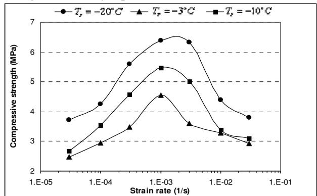
Fig. 2. Compressive strength of atmospheric ice accumulated at -10° C and tested at various temperatures. T<sub>t</sub>= Test temperature (Kermani *et al.*, 2007).
