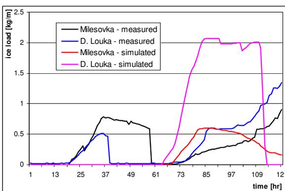
Fig. 6. Measured and simulated ice load of icing event in Jan2008 at Milešovka Mt. and Dlouhá Louka
