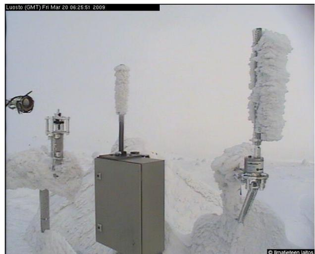
Fig. 3. Ice detectors installed at Luosto.
