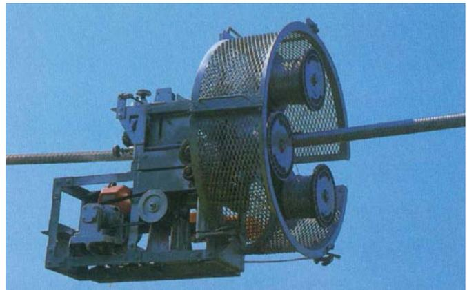
Fig. 5. Wrapping machine for the installation of LC-Spiral Rods.
