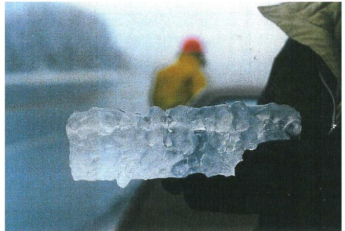
Fig. 2.6 Glaze icing sample from a conductor under test
