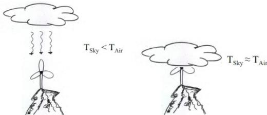
Fig. 3: Left: when the cloud base is higher than the wind turbine's nacelle, the sky temperature is significantly lower than the air temperature at the nacelle. Right: when the sky temperature is approximately equal to the air temperature, there is a high probability that the wind turbine's nacelle is in-cloud.
