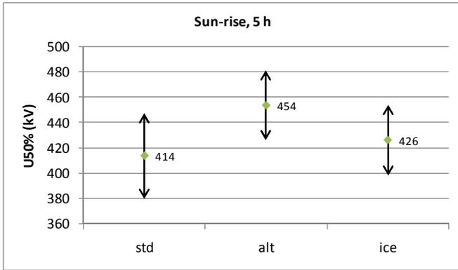
Figure 10 U<sub>50%</sub>-values derived from sun-rise tests with 5 h ice accretion. Error bars (arrows) correspond to one standard deviation.
