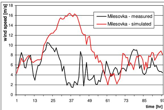
Fig. 3. Measured and simulated wind speed of icing event in 2003/04 at Milešovka Mt. The simulated wind corresponds to the lowest model layer
