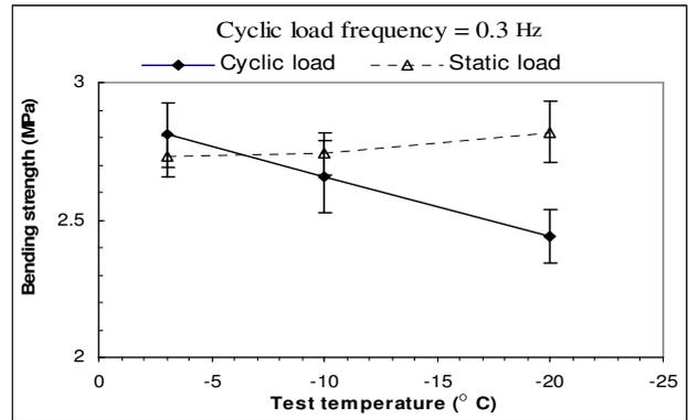
Fig. 7. Bending stress at failure for atmospheric ice accumulated at -10° C and tested at various temperatures under cyclic and static loads in the first scenario (Kermani and Farzaneh, 2009).
