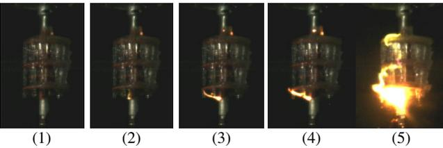
Fig.6 Flashover process of iced composite insulator polluted with solid layer method
