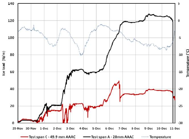
Fig. 21. Ice load in test span A with 28 mm AAAC conductor and test span C with 49.9 mm conductor during the period 29.Nov-11.Dec. 2007.
