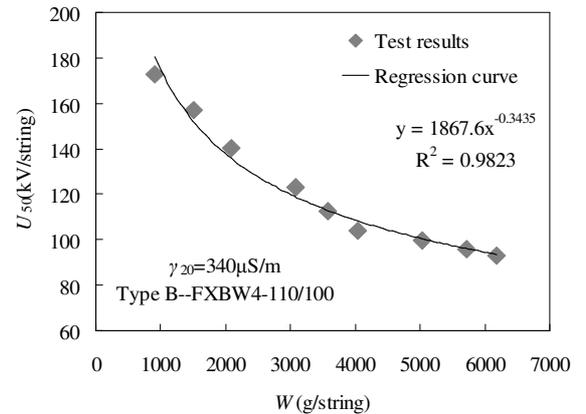
Fig.2 The relation between the  $U_{50\%}$  and ice amount
