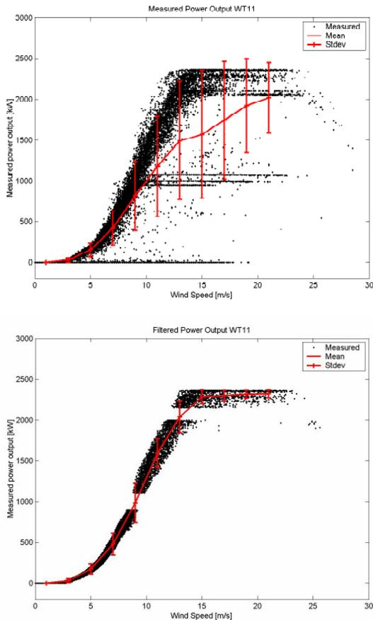
Fig. 3. French site: power output versus wind speed for wt11, all data (above) and after filtering (below).
