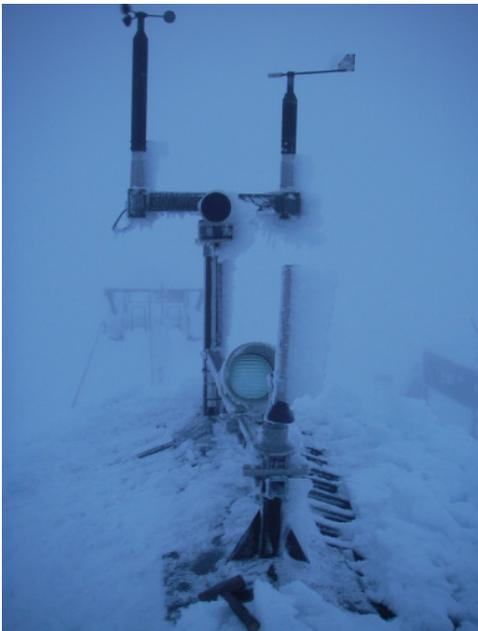
Fig. 3.2 The IceMonitor on top of the ski-house at Åre (Sweden)
