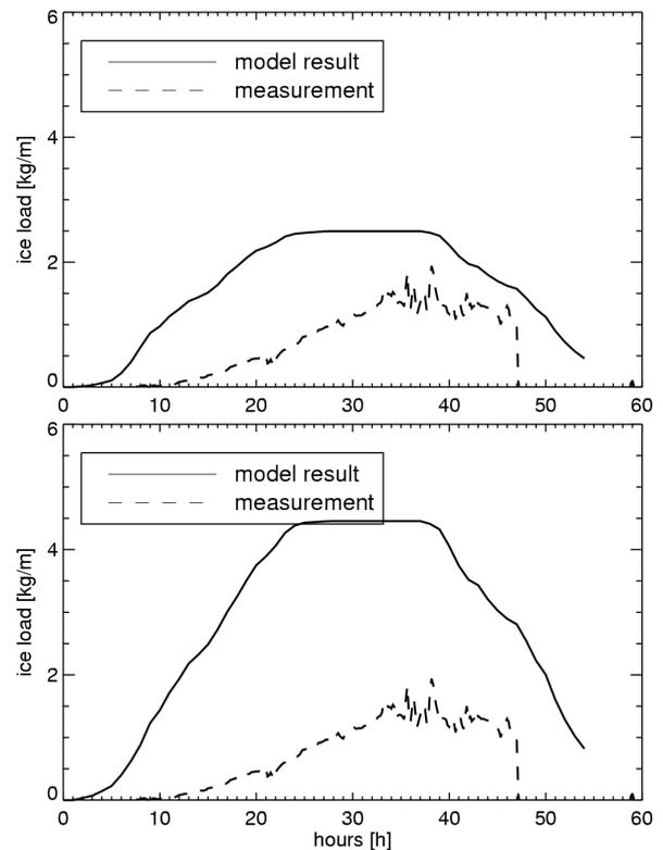
Fig. 8. Time series of simulated ice load at the position of Schwyberg for a simulation starting on 13.11..2008, 00 UTC using a volume number concentration of droplets of 300  $\text{cm}^{-3}$  in the accretion model (upper panel) and a volume number concentration of droplets of 100  $\text{cm}^{-3}$  in the accretion model (lower panel). Measurements are shown as dashed line, the model results as continuous line.
