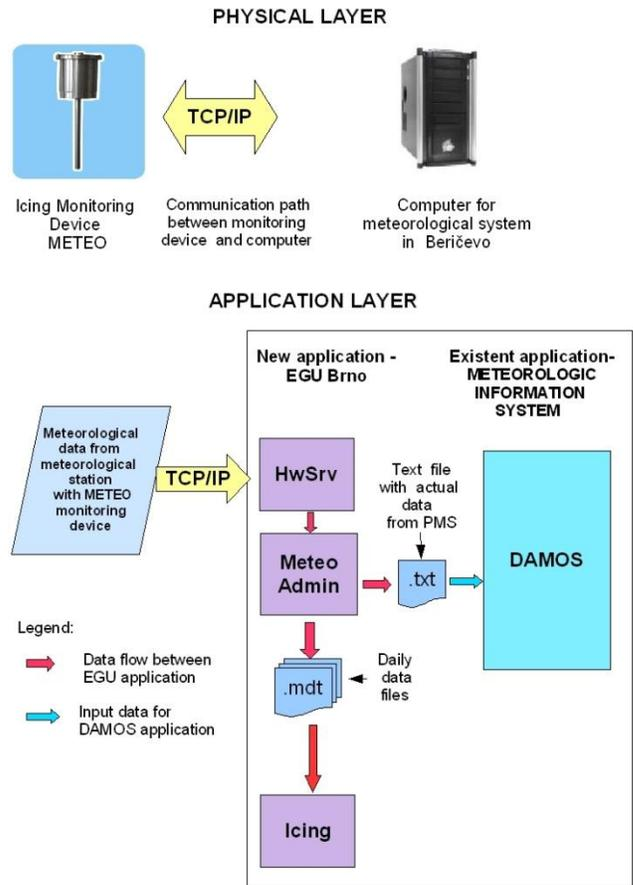
Fig. 4: Concept of ice monitoring device and DAMOS system
