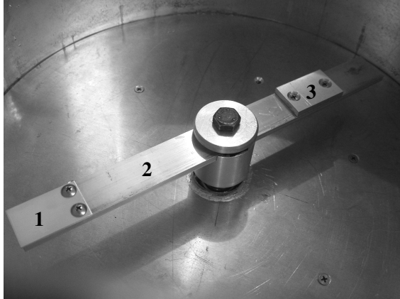
Fig. 1. Coated sample in centrifuge set-up for measuring ice adhesion. (1) Sample, (2) aluminium beam, (3) counter-weight.
