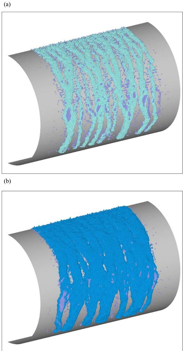
Fig. 1. Glaze ice accretion on a cylinder for a runback factor of  $\frac{3}{4}\pi$  and downstream and cross-stream motion range parameters of 2.5 and 4.5, respectively. Different colours distinguish the first and second half of the simulation.
