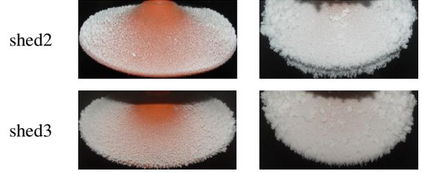
(c) Icing with energized on 20kV
