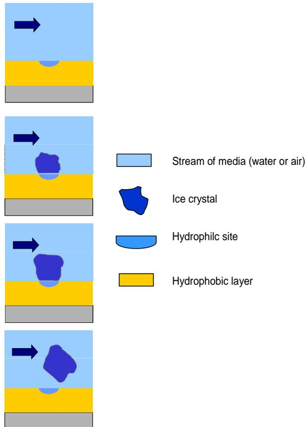
Figure 7: Scheme of hydrophobic / hydrophilic coating approach
