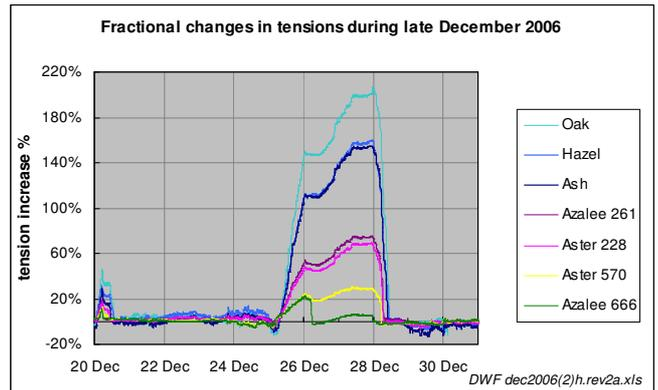
Fig. 4.2 Percentage increases in tension for conductors ranging from 14 to 31mm in diameter in December, 2006, showing the smallest conductor exceeding its design load whilst the largest conductors are hardly affected.
