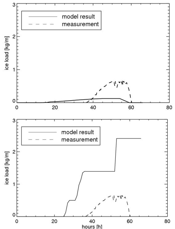
Fig. 3. Time series of simulated ice load at the position of Matzendoerfer Stierenberg for a simulation starting on 5.1.2009, 12 UTC using WRF (upper panel) and COSMO results (lower panel) as input. Measurements are shown as dashed line, the model results as continuous line.
