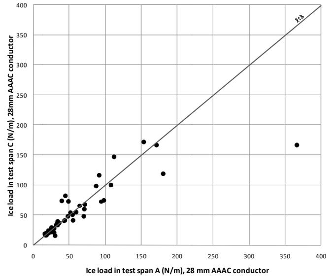
Fig. 17. Comparison between identical 28 mm AAAC conductors in test span A and test span C.
