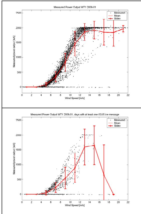
Fig. 6: Sternwald, wt1, Jan 2008, above: all data, below: data of the days when IGUS Blade Control detected ice.
