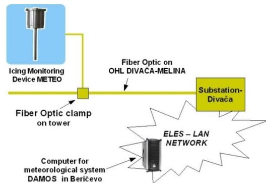
Fig. 4: Communication between ice monitoring device and main computer
