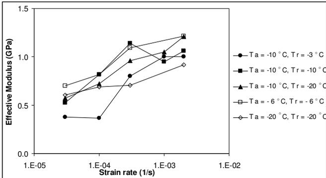
Fig. 9. Effective modulus of atmospheric ice accumulated and tested at various temperatures (Kermani *et al.*, 2008).
