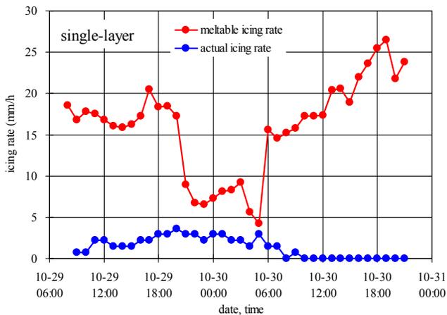
Fig. 22. Heat balance calculation results of single-layer LC-Spiral Rods
