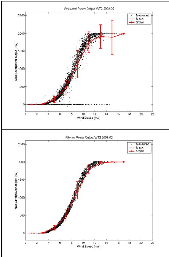
Fig. 5: Sternwald, wt2, Feb2008 data for non-icing situations, above all data, below after filtering.
