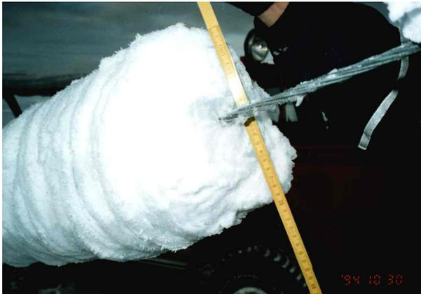
Fig. 11. In-cloud icing on guy wire in a test span at Hallormstadahals.
