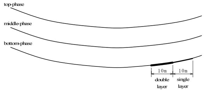
Fig. 9. Wrapping length of LC-Spiral Rods on the bottom phase conductor.
