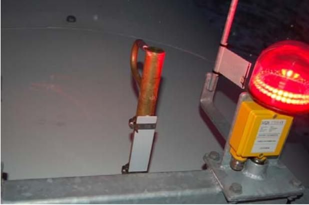
Figure 6: HoloOptics sensor installed on light boom.
