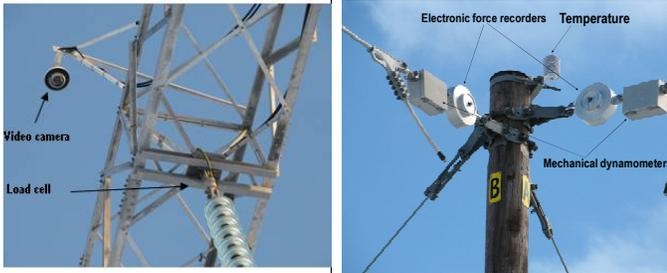
Fig. 5. Measurement equipment. OHTL to left and test span to right
