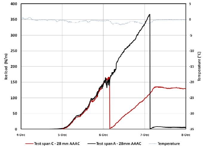
Fig. 18. Ice load in test spans A and C equipped with identical 28mm AAAC conductor in the period 4.-8. Dec.2000.
