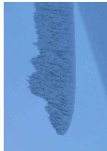
Figure 1: An iced up blade of a wind turbine in Northern Finland. The rime ice is collected on the leading edge on the left. Photo: Timo Laakso, VTT.
