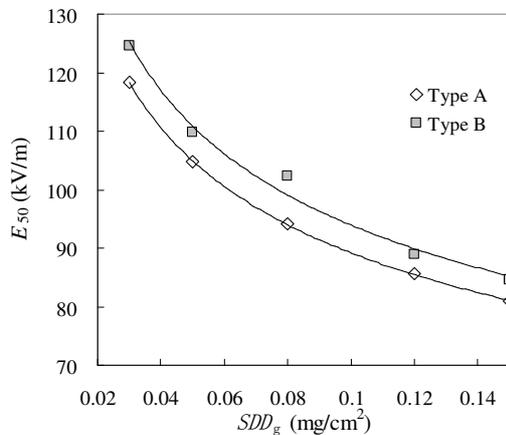
Fig.3 Flashover stress  $E_{50}$  versus  $SDD_g$
