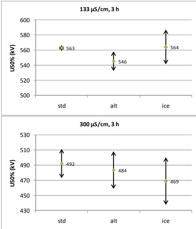
Figure 8 U<sub>50%</sub>-values derived from tests with 3 h ice accretion. Error bars (arrows) correspond to one standard deviation.
