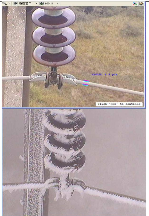
Fig.8 the normal and icing image of conductor and insulator
