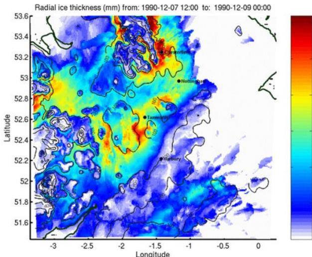
Fig. 7 Wet snow accretion on the conductors in the storm
