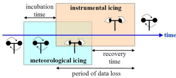
Fig. 1. Schematic representation of the different icing durations.
