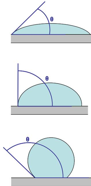
Figure 6: Principle of water contact angle with hydrophilic (left) to super-hydrophobic surface (right)
