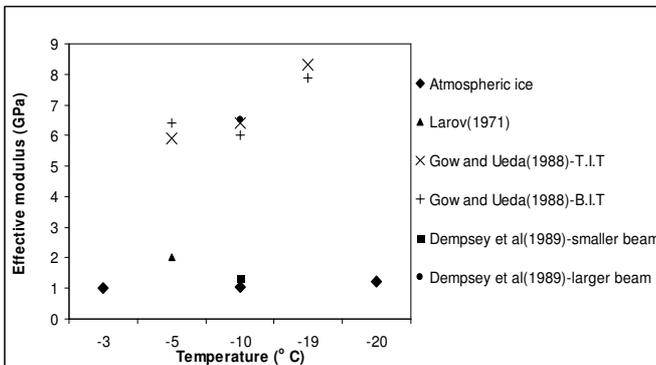
Fig.10. Comparison of effective modulus of atmospheric ice with values of other researchers for fresh water ice (T.I.T= Top In Tension; B.I.T= Bottom In Tension) (Kermani *et al.*, 2008).
