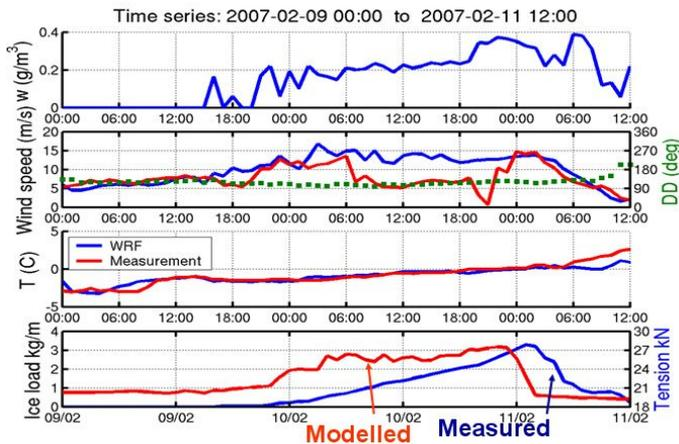
Fig. 2 Measured and modeled data for Deadwater Fell. Red lines are measured data and blue lines are modeled values. Green squares illustrate simulated wind direction.
