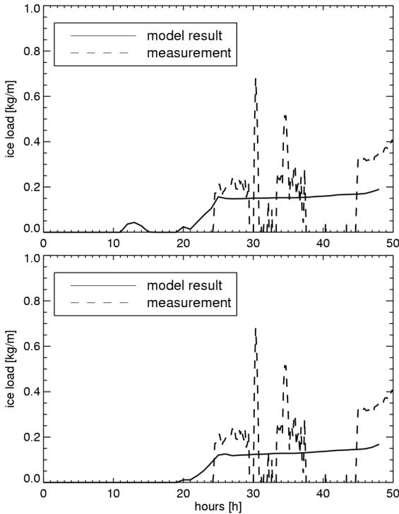
Fig. 10. Time series of simulated ice load at the position of Schwyberg for a simulation starting on 27.03..2009, 12 UTC using a volume number concentration of droplets of  $100 \text{ cm}^{-3}$  in the WRF model (upper panel) and a volume number concentration of droplets of  $300 \text{ cm}^{-3}$  in the WRF model (lower panel). Measurements are shown as dashed line, the model results as continuous line.
