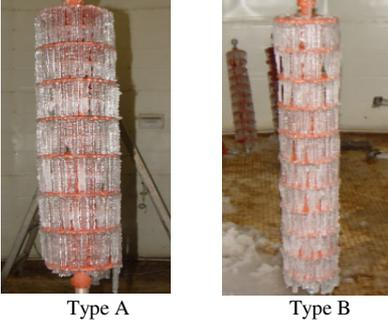
Fig.8 photos of ice-covered tested insulators
