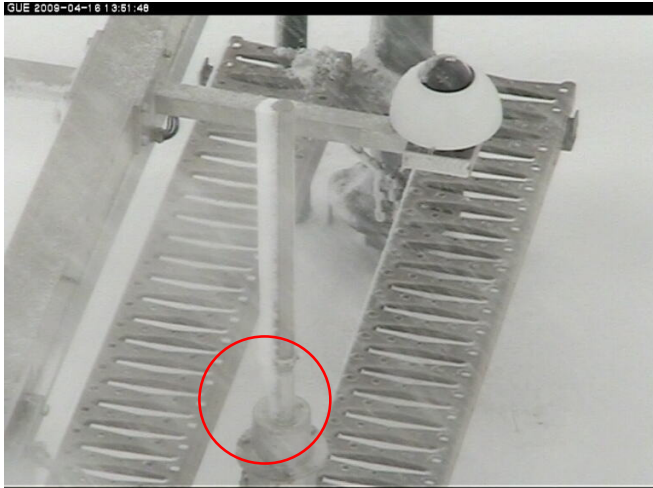
Picture 2: April 16 th , 15h, snow bridge prevents rod rotation of Combitech IceMonitor
