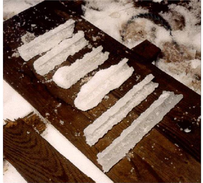
Fig. 2.5 Ice accretion samples from different conductors on test at Deadwater Fell.
