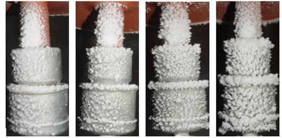
(a) Non-energized (b)10kV (c)20kV (d)30kV
