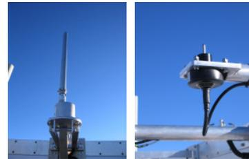
Fig. 4: Left: Combitech IceMonitor, right: Goodrich Ice Detector.
