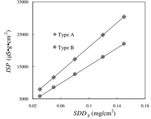
Fig9 The relation curve between  $SDD_g$  and  $ISP$
