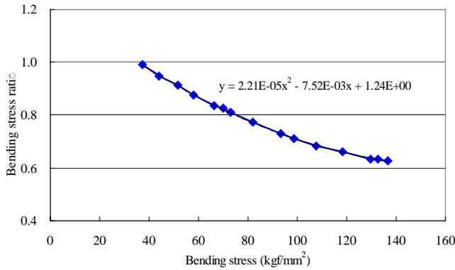
Fig. 11 Bending stress ratio of the new lightweight interphase spacer (Linear - Nonlinear)
