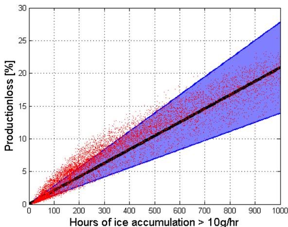
Fig. 7. Production loss estimate for Nordland. The red dots represent calculations from individual grid cells using time series of wind speed and icing.
