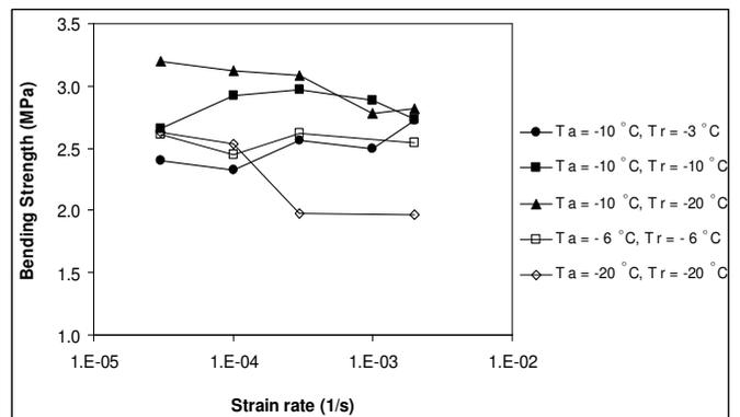
Fig.5. Bending strength of atmospheric ice accumulated and tested at various temperatures (Kermani *et al.*, 2008).
