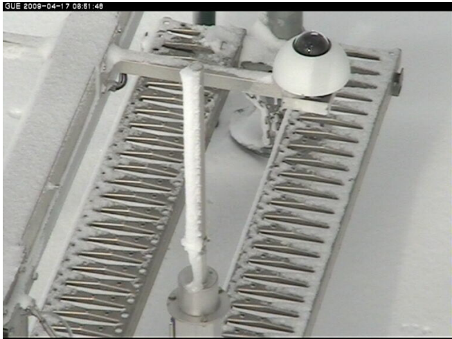
Picture 3: April 17 th , 8h, free rotation of Combitech IceMonitor
