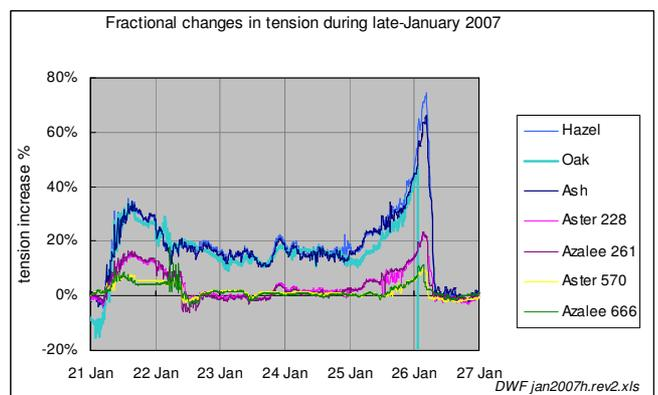
Fig. 4.3 Percentage increases in tension for conductors ranging from 10 to 31mm in diameter. The severe effect of wind/ice incidents on small conductors can clearly be seen
