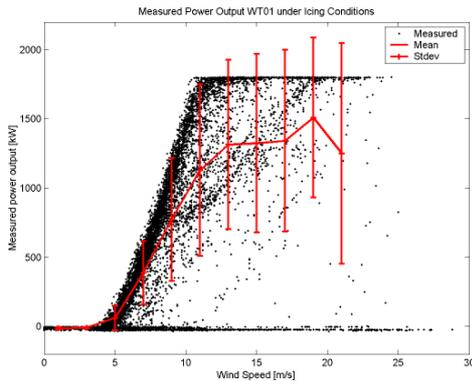
Fig. 8. Power output wt01 under icing conditions.
