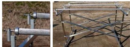
Figure 4: the test-conductors was built by TTD Laboratory: conductors have a steel core with aluminum coating (ACSR). Wires are not current supplied.
