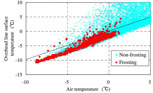
Fig. 8. Relationship between air temperature and overhead line surface temperature. Solid line shows that air temperature is equal to the overhead line surface temperature.
