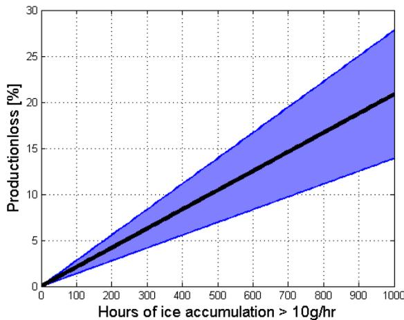
Fig. 6. Estimated range for production loss. Lower boundary is given by (2). Upper boundary is given as twice the lower boundary.
