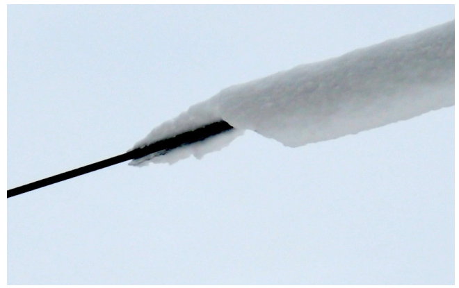
Fig. 1. Cylindrical wet-snow accretion on a conductor. Source: E.ON Northwestern Hungary Electricity Supplying Zrt. (9th of February, 2009., Bakony)
