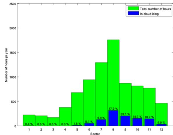
Fig. 5. Distribution of wind direction for a site in Nordland. The green bars represent the distribution for all data at this point. The blue bars represent the wind direction for the cases where the icing rate exceeds 10 g/hr. The magnitude of the blue bars relative to the green bars is given as percentage. The distribution is given as 12 sectors, where sector 1 represents northerly wind.
