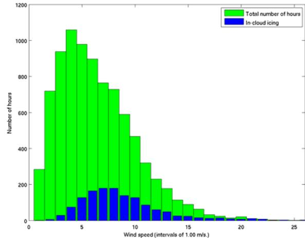
Fig. 4. Wind speed distribution for an exposed site in Nordland. The green bars represent the distribution for all data at this point. The blue bars represent the distribution in wind speed for the cases where the icing rate exceeds 10 g/hr.
