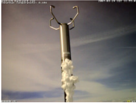
Left: image of Thies Ultrasonic anemometer on nacelle of the wind turbine. Right: image of rotor blade.
