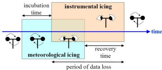
Fig. 2: Meteorological and Instrumental Icing.
