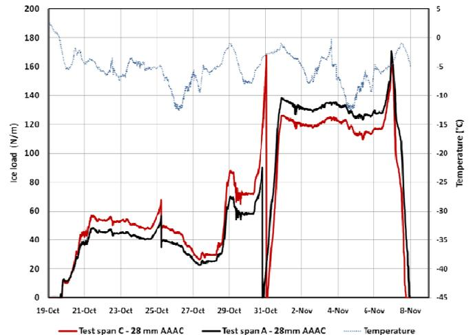
Fig. 19. Ice load in test spans A and C equipped with identical 28mm AAAC conductor during the period 19.Oct.-08 Nov.2005.
