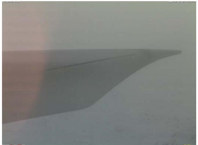
Figure 5: Icing indicated by HoloOptics, but fog and low light makes it impossible to detect icing visually.
