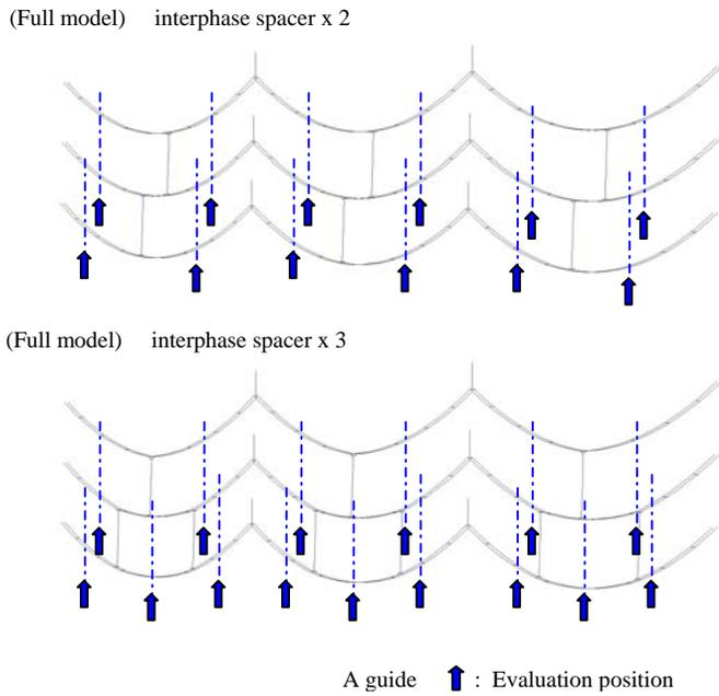
Fig. 3 Evaluation position in analytical model
