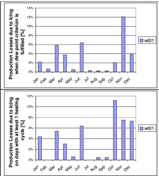
Fig. 9: Production losses due to icing above: when the dew point criterion is fulfilled, below on days with at least one heating cycle.
