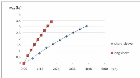
Fig. 11. Mass of dripping water as function of sleeve length
