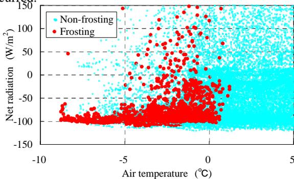
Fig. 7. Relationship between air temperature and net radiation
