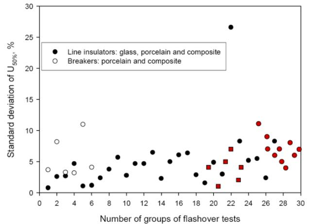
Figure 5 Standard deviations of flashover voltages generally below 10% [7]. Red circles and squares indicate results of measurements made within this project (5 and 3 hours of ice accretion respectively).
