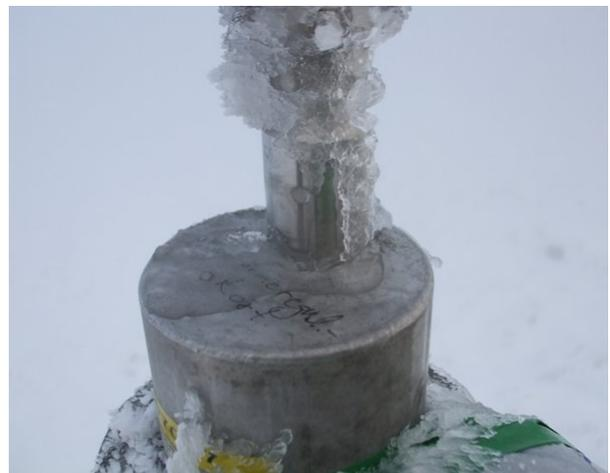
Fig. 4.1 Ice bridging the Combi-Tech rod and base.
