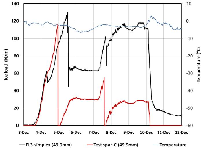
Fig. 27. Ice load with 49.9 mm AACSR conductor in FL3 (400 kV OHTL) and test span C during the period 3-12 Dec. 2006.
