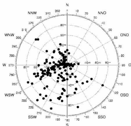
Fig. 5: Distribution of ice throw around the turbine.
