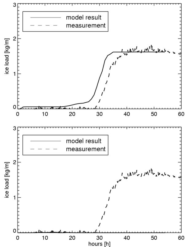
Fig. 6. Time series of simulated ice load at the position of Guetsch for a simulation starting on 22.11.2007, 00 UTC using WRF results at 800 m grid size (upper panel) and at 3.2 km grid size (lower panel) as input. Measurements are shown as dashed line, the model results as continuous line.
