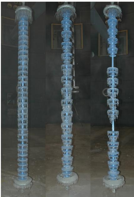
Figure 3 Insulators after test with 3 hours of ice accretion time. From left to right: standard profile, alternating profile and ice-breaker profile.
