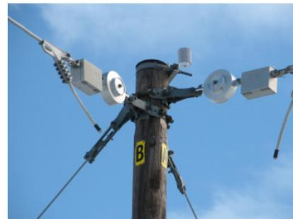
Fig. 6. Test Span Load Cell and Data Logger Detail [43].
