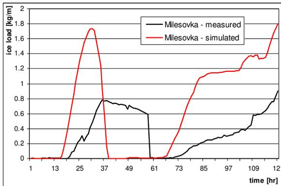
Fig. 8. Measured and simulated ice load of icing event in Jan2008 at Milešovka Mt. after adiabatic correction
