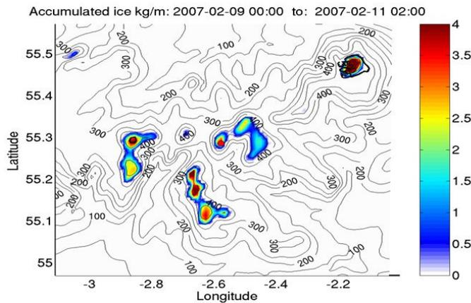
Fig. 3 Accumulated ice load data according to geographical location. Area shown is Scottish Borders with Deadwater Fell at 55.3 Latitude and -2.6 Longitude.
