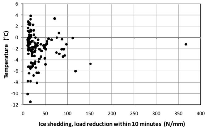
Fig. 8. Ice shedding in test span A, period 1997-2009.
