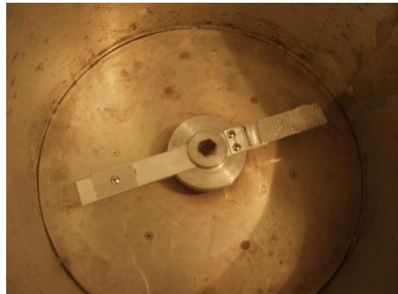
Fig. 3. The centrifuge machine
