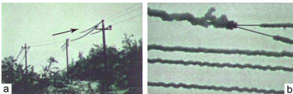
Fig. 2 Creep of a wet snow sleeve on a steep cable (from [3])
