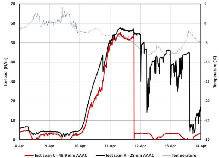
Fig. 23. Ice load in test span A with 28 mm AAAC conductor and test span C with 49.9 mm conductor during the period 9-14 Apr. 2009.
