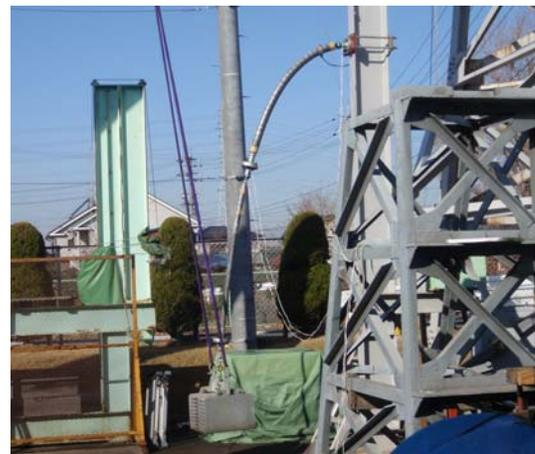
Fig. 9 The bend test of the new lightweight interphase spacer
