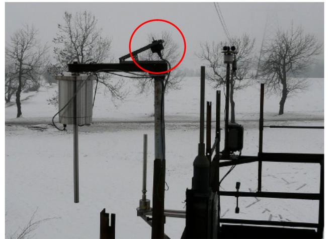
Fig. 5 Ice detector Goodrich and METEO on the platform at 10 m
