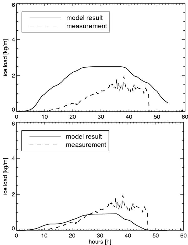
Fig. 7. Time series of simulated ice load at the position of Schwyberg for a simulation starting on 13.11..2008, 00 UTC using WRF results at 800 m grid size (upper panel) and at 3.2 km grid size (lower panel) as input. Measurements are shown as dashed line, the model results as continuous line.
