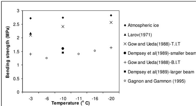
Fig.6. Comparison of bending strength of atmospheric ice with values of other researchers for fresh water ice and glacier ice (T.I.T= Top In Tension; B.I.T= Bottom In Tension) (Kermani *et al.*, 2008).
