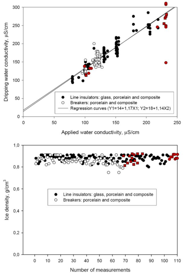
Figure 4 Relation between dripping- and applied water conductivities (top) and recorded ice densities of about 0,90  $\text{g}/\text{cm}^3$  (bottom) [7]. Red circles and squares indicate results of measurements made within this project (5 and 3 hours of ice accretion respectively).
