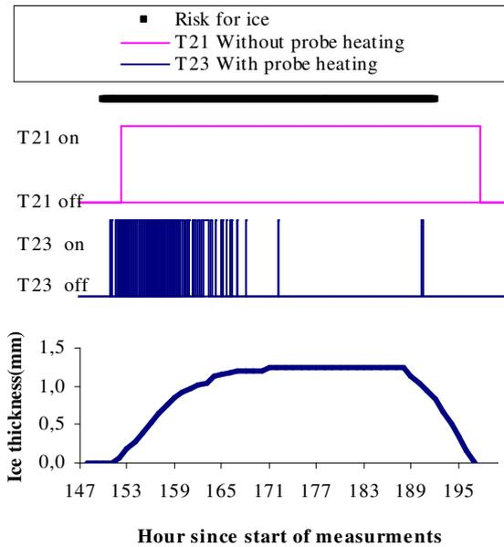
Fig 1 Example of indications and calculated ice thickness
