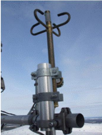
Fig. 5.3 The HoloOptic icemeter at Deadwater Fell
