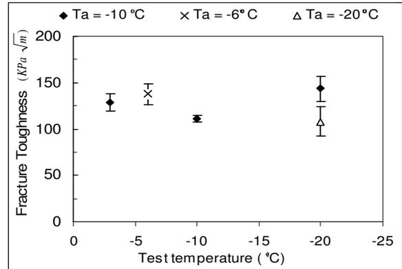
Fig. 11. Fracture toughness of various types of atmospheric ice. The error bars in this figure correspond to the standard error in the results for the tests conducted with each set of parameters (Kermani & Farzaneh, 2008).
