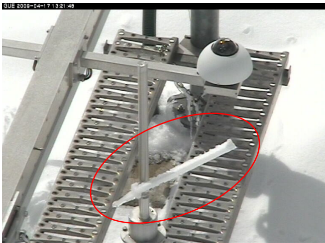
Picture 4: April 17 th , 14h30, release of Combitech IceMonitor
