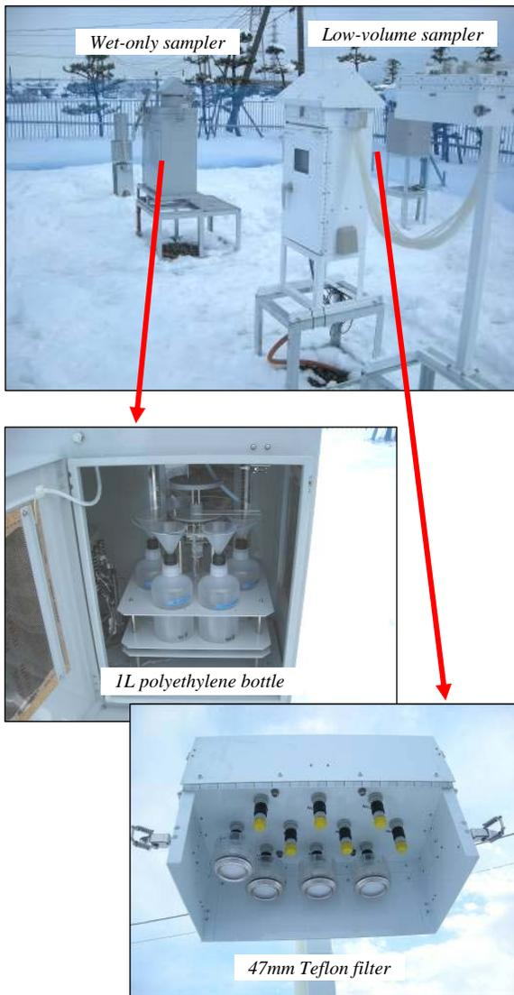
Fig. 2. Wet-only sampler for collecting snow samples and Low-volume sampler for collecting atmospheric aerosol samples
