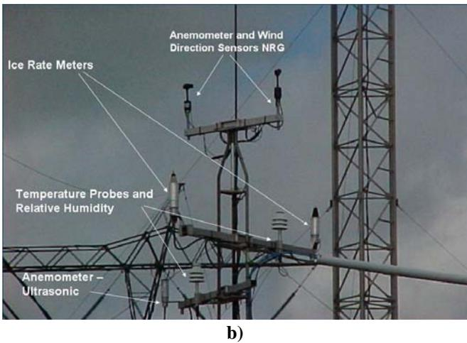
Fig. 11. a) Sketch of the Mont Bélair icing test site and measuring equipment; b) Photo of meteorological instruments at Mont Bélair.
