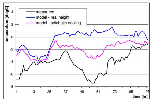
Fig. 7. Measured temperature  $T_m$ , output from the model level  $T_{lev}$  and temperature of lifted air  $T$  during icing event in Dec2007 at Milešovka Mt.
