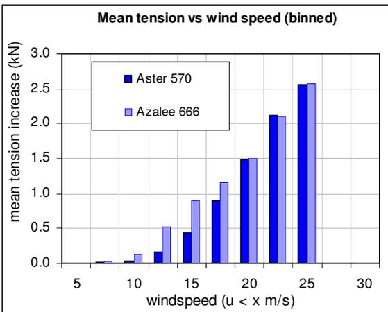
Fig. 4.5 Effect of wind only (no ice) on smooth (light blue) and stranded (dark blue) conductors of 31mm diameter
