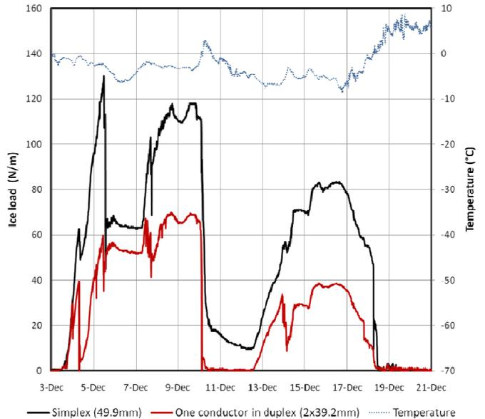
Fig. 15. Ice load on simplex conductor (49.9 mm) and one sub-conductor in a duplex conductor (2x39.2 mm) during the period 3-21 Dec. 2006.
