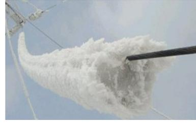
Fig.1 Photo of cylindrical glaze ice on transmission line
