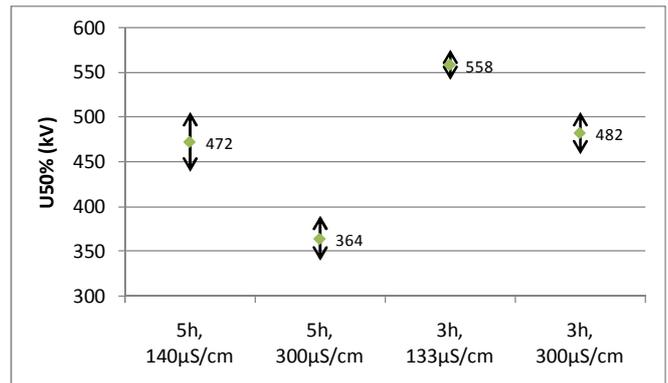
Figure 9 Average U<sub>50%</sub>-values per test condition. Error bars (arrows) correspond to one standard deviation.
