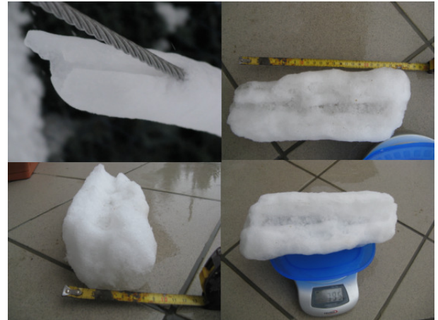
Fig. 14. The estimated wet-snow load was heavier than 4-5 kg/m in this case. Source: E.ON Northwestern Hungary Electricity Supplying Zrt. (28th of January, 2009)
