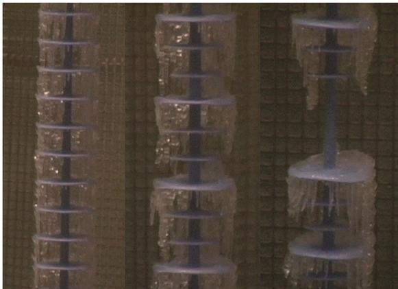
Figure 2 Detail of mid portion of insulators with ice after 5 hours of ice accretion, i.e. exposure to water spraying (from left to right: standard, alternating and ice-breaker profile).
