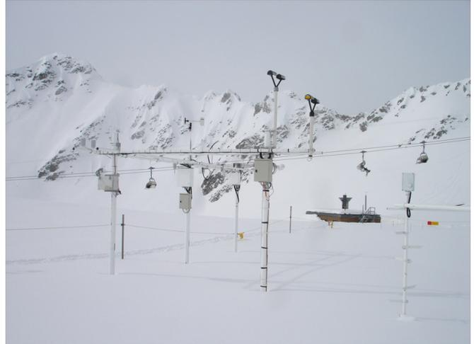
Fig. 3. The 2 Parsivel optical disdrometers deployed at the Weissfluhjoch site (and other instruments).
