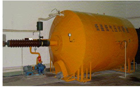
Fig.1. Artificial climate chamber of Chongqing University
