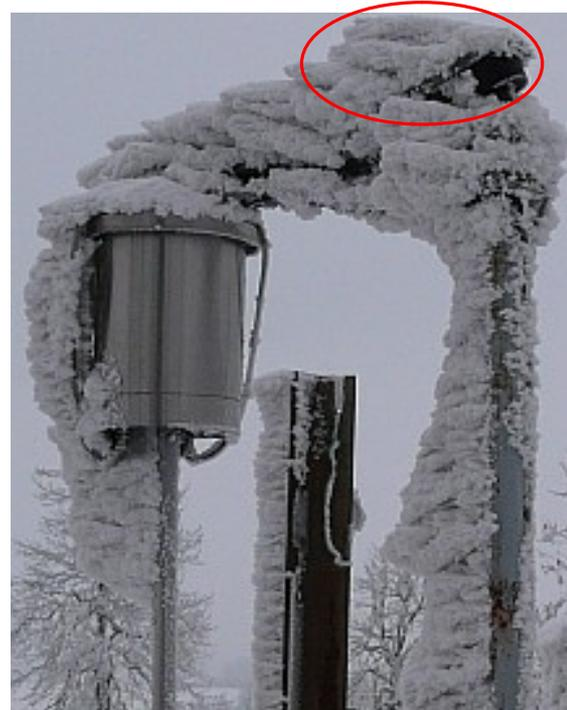
Fig. 7 Ice detector Goodrich fully covered with ice
