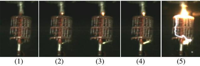
Fig.7 Flashover process of iced composite insulator polluted with icing-water-conductivity method
