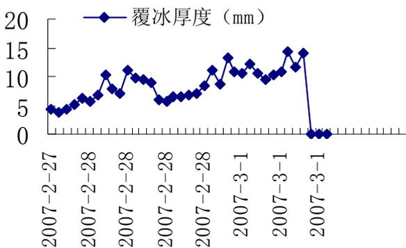
Fig. 3 The development process of the icing from February 27 to March 1 2007
