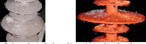
Fig.5 photos of water droplets and ice particles on the surface of composite insulators
