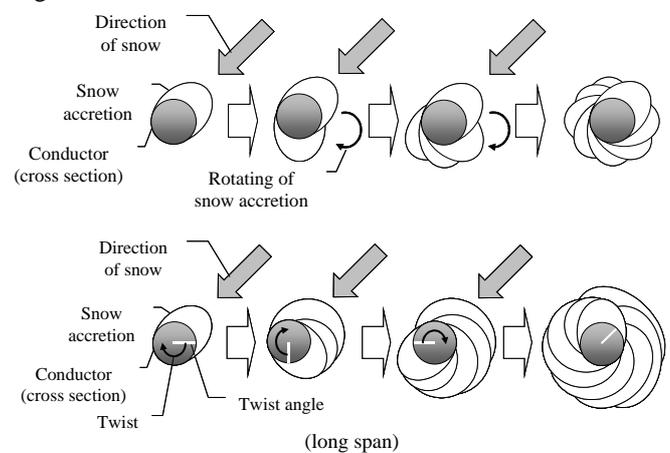
Fig. 1. Process of snow accretion (wet snow) on a small conductor
