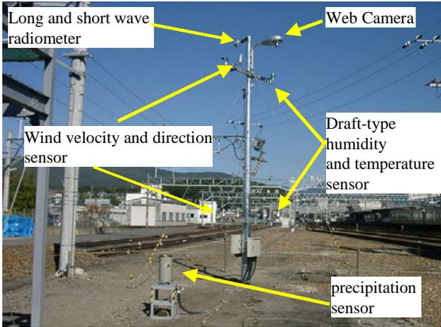
Fig. 2. Establishment situation of weather surveying instruments
