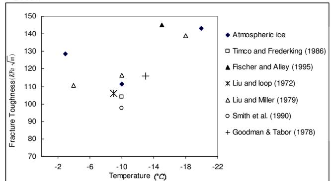
Fig. 12. Comparison of fracture toughness of ice with the results of other research on fresh water ice (Kermani & Farzaneh, 2008).
