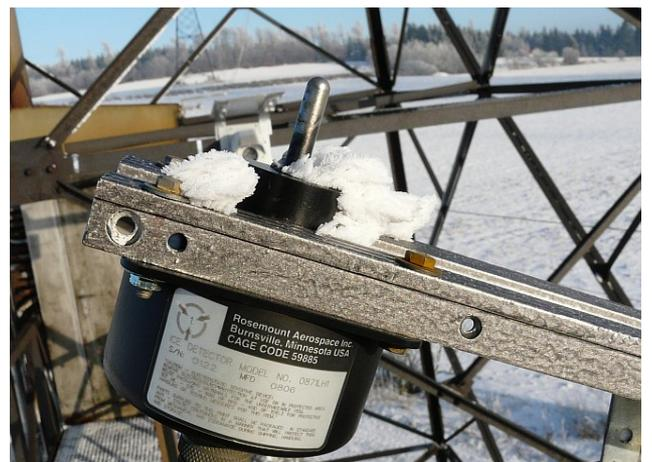
Fig. 6 Ice detector Goodrich in detail
