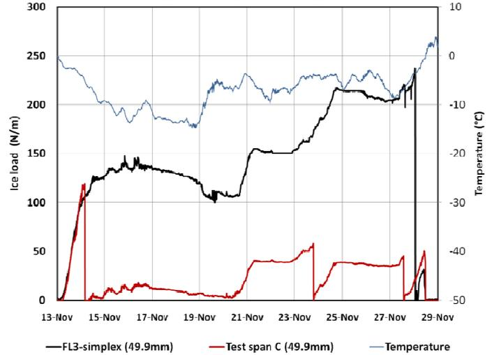
Fig. 26. Ice load with 49.9 mm AACSR conductor in FL3 (400 kV OHTL) and test span C during the period 13-29 Nov. 2006.
