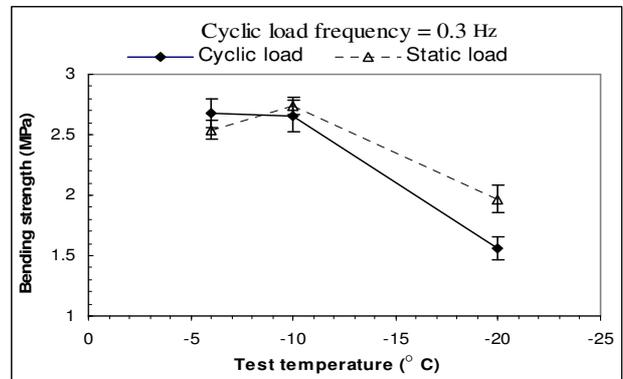
Fig. 8. Flexural strength of atmospheric ice accumulated and tested at various temperatures under cyclic and static loads in the first scenario (Kermani and Farzaneh, 2009).
