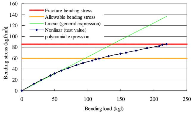
Fig. 10 Bending loading - Bending stress characteristic of the new lightweight interphase spacer (Linear - Nonlinear)
