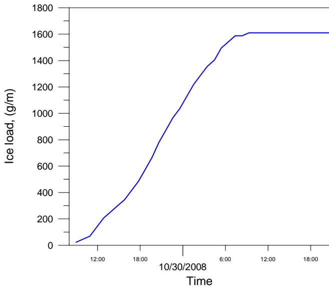
Fig. 20. Ice load evaluated by the Ice Rate Meter as a function of time.
