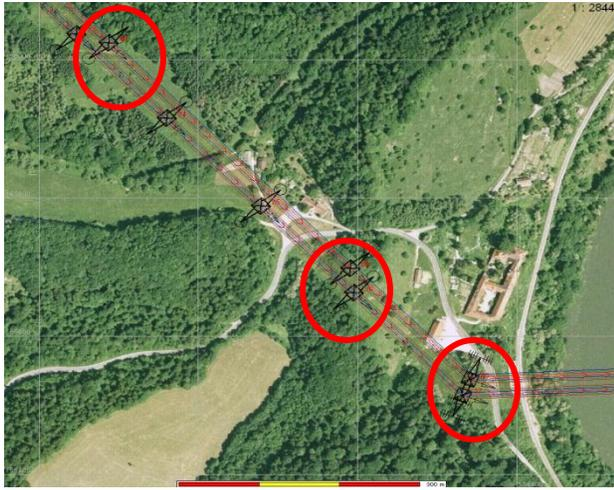
Fig. 8: Situation of collapsed towers of double circuit 110 kV OHL in Northern part of Slovenia on January 28, 2009
