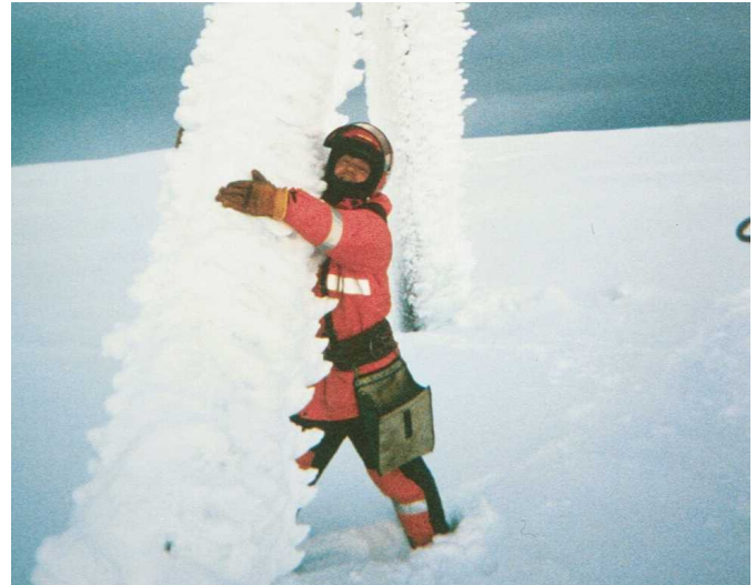
Fig. 5. In-cloud icing on a test span close to shore, 650 m a.s.l.
