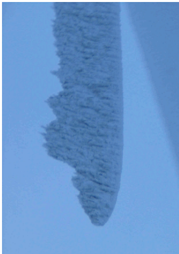
Figure 2: An iced up blade of a wind turbine in Northern Finland. The rime ice is collected on the leading edge on the left. Photo: Timo Laakso, VTT.
