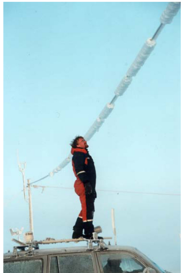
Fig. 4. A triangular test span (73-4), in-cloud icing on span 73-4-A.
