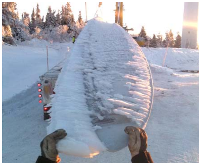
Figure 3: Ice collected on a wind turbine blade.
