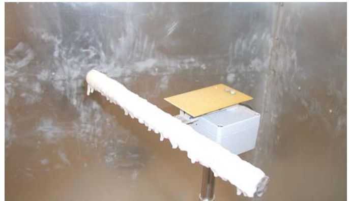
Fig. 8. Experimental investigations of monitoring system in climatic cell
