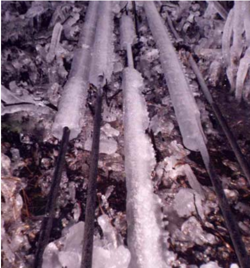
Fig. 6. Icing on OHL 750 kV conductors: a) Isakcha - Yuzhnoukrainskaya
