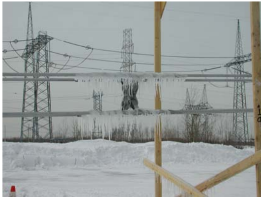
Fig. 8. Ice retention effect of spacer and tie rods
