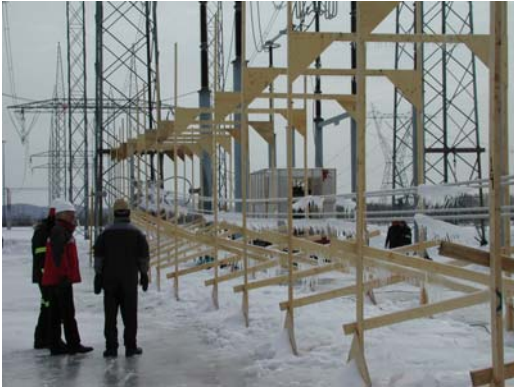
Fig. 7. Outdoor de-icing test on a 80 meters 735-kV 4 conductors bundle span equipped with 2 spacers
