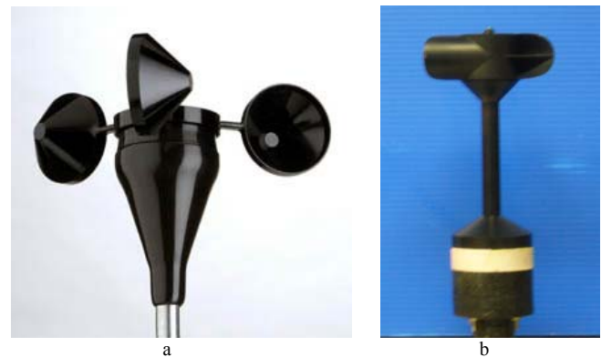
Fig. 1. Cup anemometers: a) NRG#40 and b) NRG first generation Ice-free Electrically Heated Anemometer.
