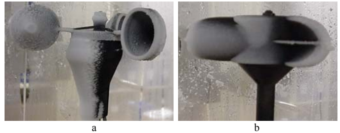
Fig. 4. Iced cups at 10 m/s after 60 min a) NRG#40 and b) NRG first generation Ice-free Electrically Heated Anemometer.
