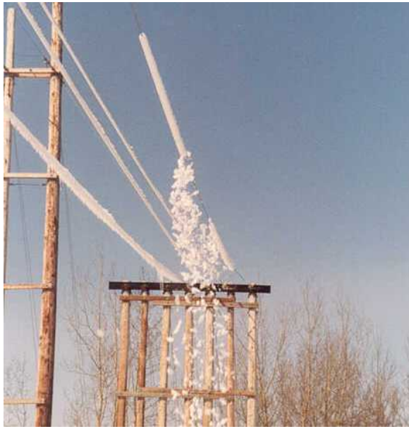
Photo 4 Pieces of ice falling to the ground during the second and final twisting sequence (February 2003 de-icing test)
