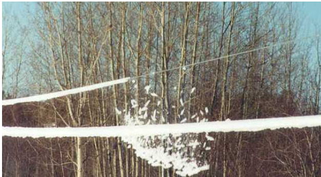
Photo 5 Pieces of ice removed during the first twisting sequence (March 2003 de-icing test)
