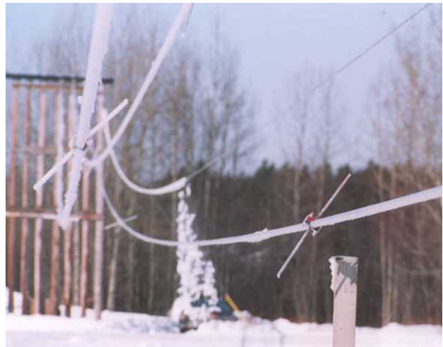
Photo 3 Pieces of ice falling to the ground following three cable rotations. (February 2003 de-icing test)
