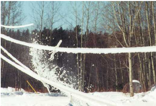
Photo 6 Same as Photo 5, but a few turns later (March 2003 de-icing test)
