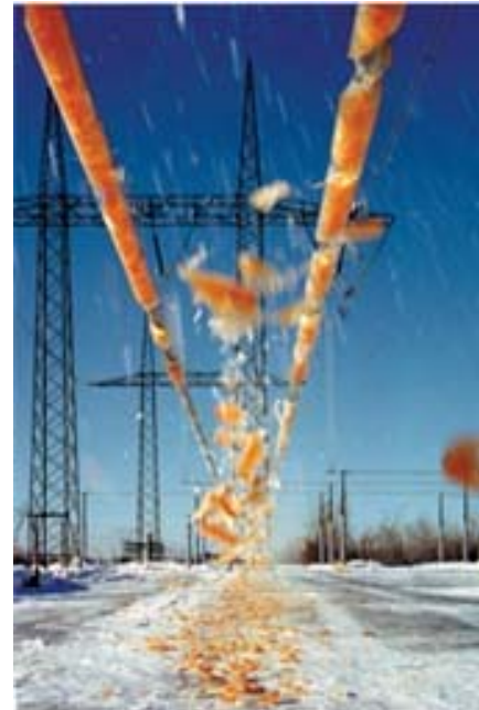
Fig. 1. De-icing a twin bundle using 10 kA and an appropriate reclosing sequence. Reference [19].
