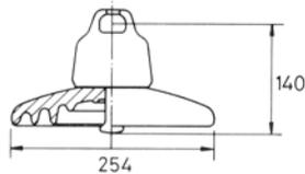
Fig. 6. Sample disk of porcelain suspension insulator
