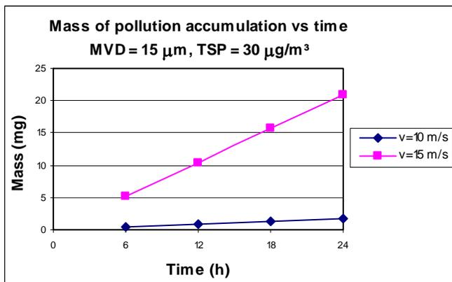
Fig. 10. Mass of pollution accumulation versus contamination event duration at different wind speed
