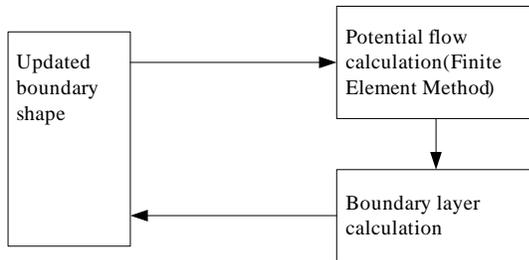
Fig. 3. Airflow computation
