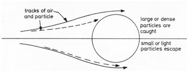
Fig. 2. The air flow field about an object
