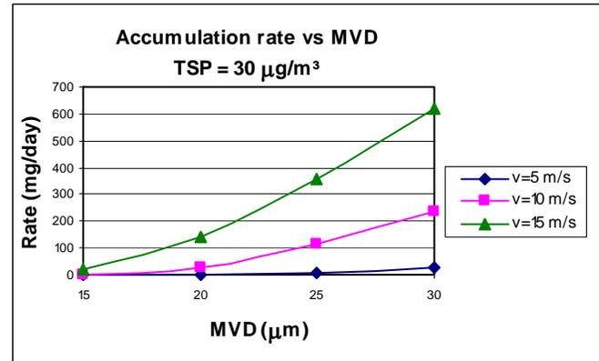
Fig. 8. Accumulation rate versus MVD at different wind speed
