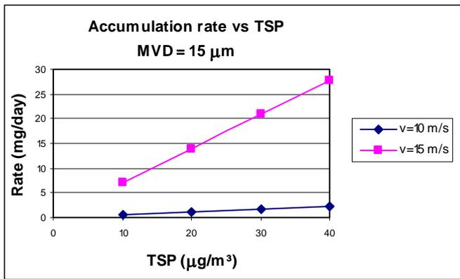
Fig. 9. Accumulation rate versus TSP at different wind speed
