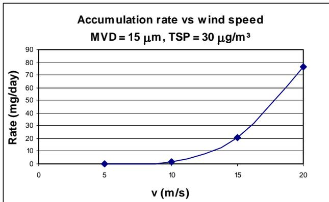
Fig. 7. Accumulation rate versus wind speed
