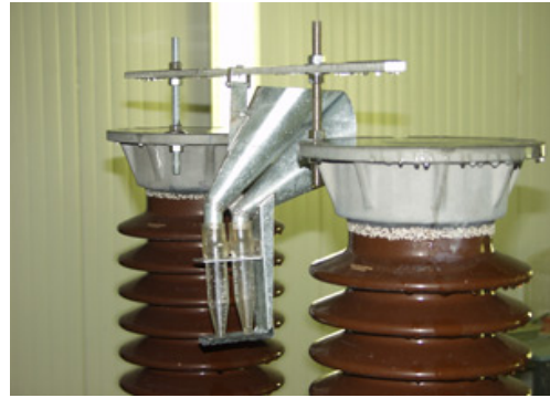
Fig. 3. Standard device for precipitation rate measurements
