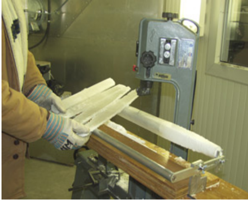
Fig. 5. Thick section preparation using a band saw
