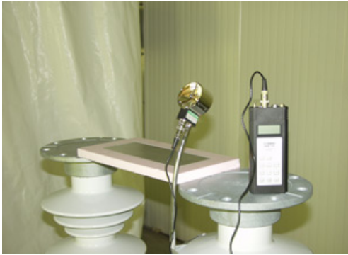
Fig. 1. Insulated aluminum-plate and air-speed anemometer
