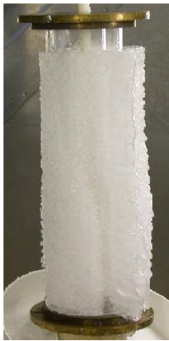
Fig. 1: Ice sample and flashover test set-up.
