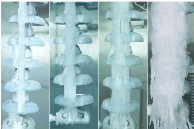
Fig. 9: IEEE standard insulator string with different ice layer width to simulate effects of insulator diameter
