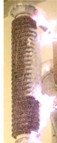
Fig. 3: Flashover on post type insulators
