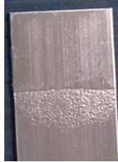
Figure 9 – Photograph of the aluminum beam test surface following a centrifuge test. Note, the ice block is entirely removed indicating an adhesive failure
