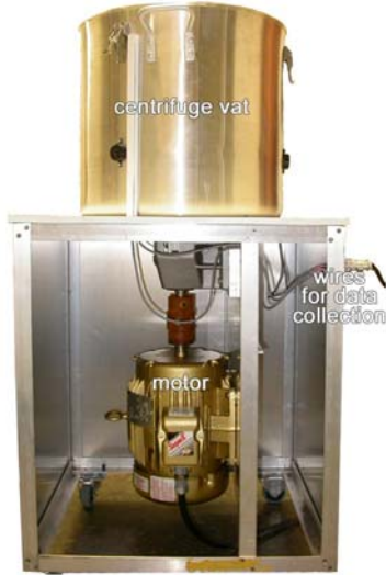
Figure 6 – Centrifuge test set-up, contained in the cold room of Figure 4.
