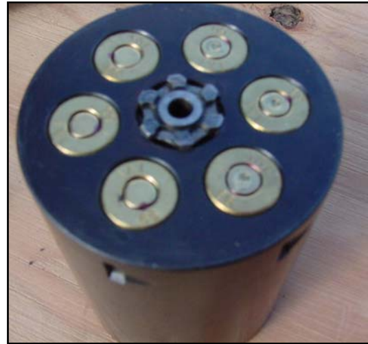
Fig. 3. Barrel of the revolver system stocking 6 blank cartridges.
