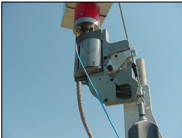
Fig. 2. Revolver system with solenoid for multiple firings.
