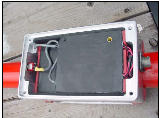
Fig. 4. Encapsulated electronic circuit receiver inside the aluminum box.
