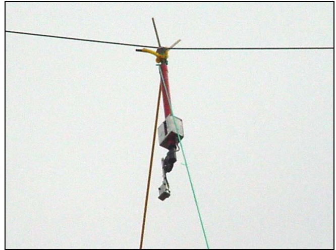
Fig. 7. DAC held in place by a taut rope and ready to be fired.
