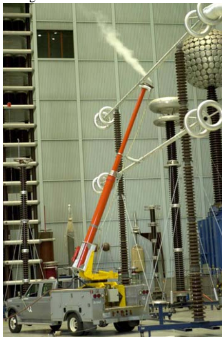
Figure 5: Dielectric tests (prototype)
