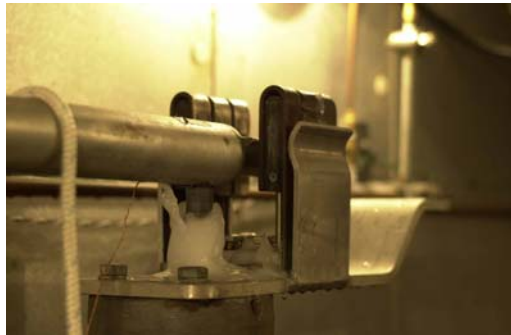
Figure 1b: Jaw de-iced using steam
