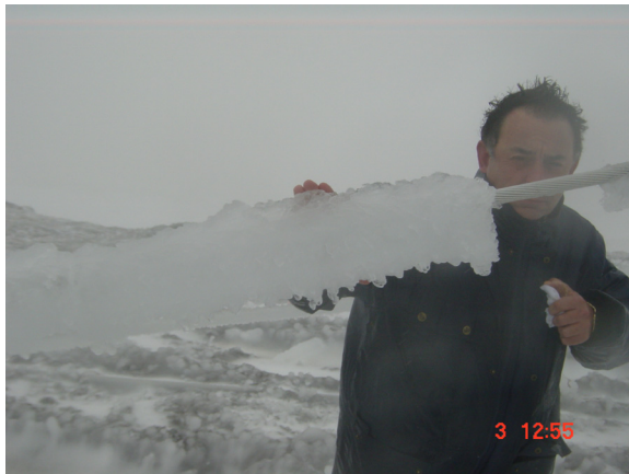
Fig. 2. Icing on a power line in Spain January 2004 (Photo: Iberinco).
