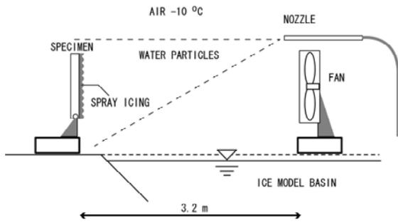
Fig. 2. Apparatus on an ice model basin.
