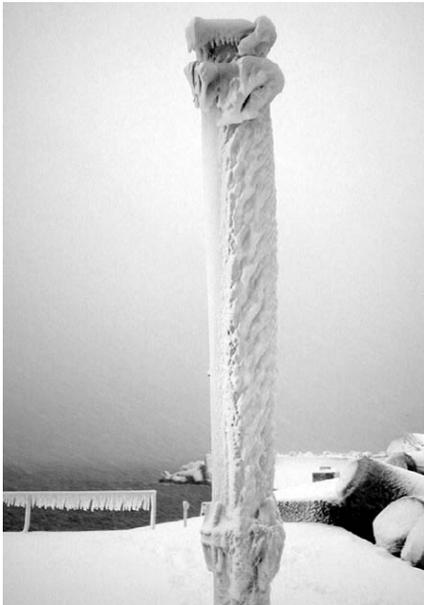
Fig. 9. Sea spray icing on steel dummy lighthouse.
