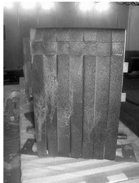
Fig. 4. Spray icing on fiber reinforced plastic belt.
