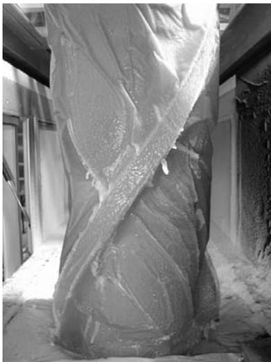
Fig. 7. Spray icing on waterproof nylon cloth with spiral-shaped spacer.
