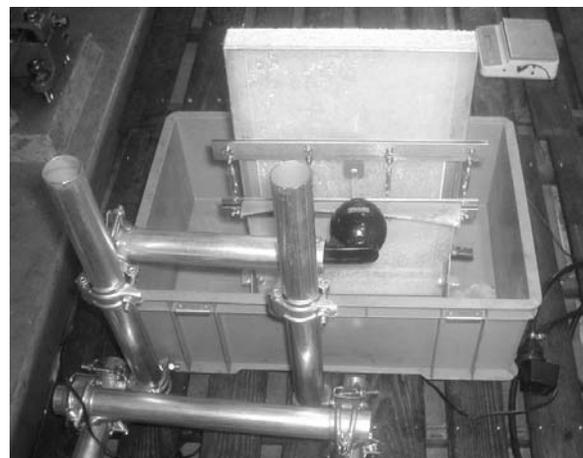
Fig. 5. Vibration test of ice accreted film specimen.
