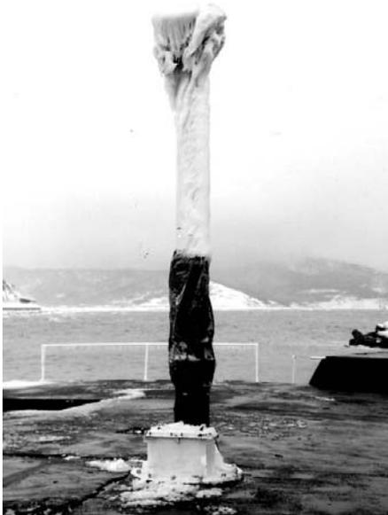
Fig. 10. Anti-icing effect of membrane structure.
