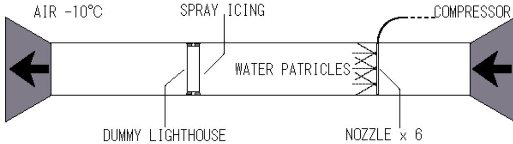
Fig. 6. Schematic view of wind tunnel test.
