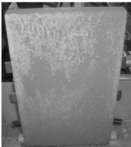
Fig. 3. Spray icing on polyester coated with vinyl chloride.
