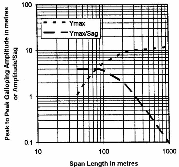
Fig. 9. Peak to peak galloping amplitude and peak to peak galloping amplitude divided by sag as a functions of span length for single conductors [16]
