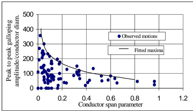
Fig. 10. Variation of observed maximum peak to peak galloping amplitude / diameter on single conductors as a function of the conductor span parameter [17]
