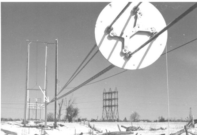
Fig. 1. Outdoor test line at Ontario Hydro used for bundle torsional stability studies showing twisted sub-conductors in mid-subspan (arrow) following collapse [7]
