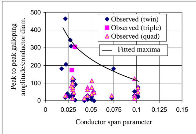
Fig. 11. Variation of observed maximum peak to peak galloping amplitude / diameter on bundle conductors as a function of the conductor span parameter
