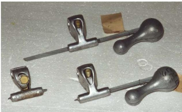
Fig. 4. Failed Stockbridge type dampers damaged by low frequency aeolian vibration of conductors covered with hoar frost
