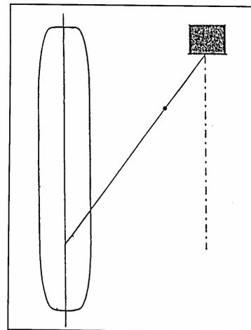
Fig. 12. Proposed modified galloping motion envelope based on analysis of films of observed galloping occurrences [15]
