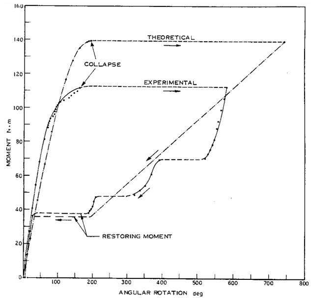
Fig. 2. Measured and theoretical values of applied moment versus angular rotation for a torsional stability test on a two conductor bundle [7]
