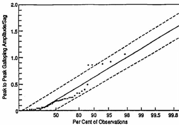
Fig. 7. Peak to peak galloping amplitudes of large single conductors without galloping controls from field observations during 43 different galloping events. Values normalized by dividing by sag [15]
