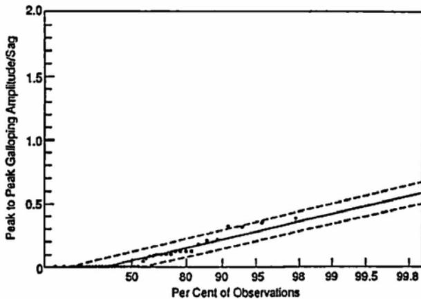
Fig. 8. Peak to peak galloping amplitudes of large single conductors with detuning pendulums from field observations during 43 different galloping events. Values normalized by dividing by sag [15]
