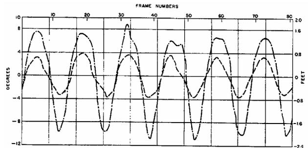
Fig. 5. Vertical and torsional galloping motions from frame by frame analysis of movie film of a single conductor span with midspan target. - - - - vertical - - - - torsional, horizontal scale 0.5 sec. intervals
