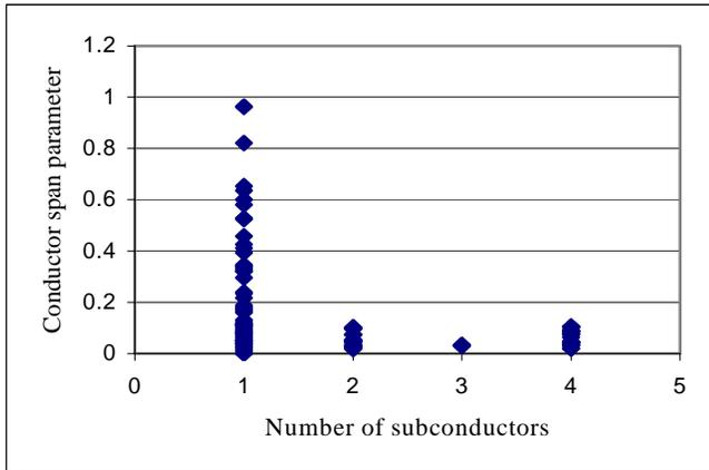
Fig. 13. Conductor span parameter as a function of number of subconductors. This shows a clear distinction between single and bundle conductors, and the similarity among all types of bundle conductor [17]
