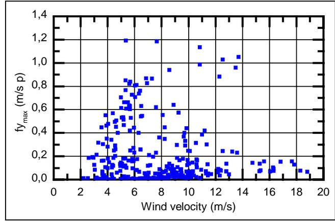
Fig. 10:  $f_{y_{max}}$  at 41% RTS after 38 days of the first galloping test
