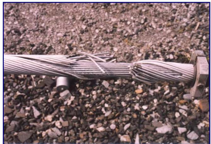
Fig. 12: Damaged conductor under the metal-to-metal clamp in the 450-m span after six days of the second galloping test
