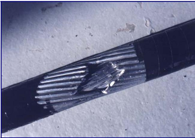
Fig. 15: Damaged conductor under the metal-to-metal clamp in the 450-m span at the end of the second test
