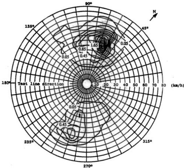
Fig. 4: Maximum values of the subspan oscillation instability index of a quad bundle [7]
