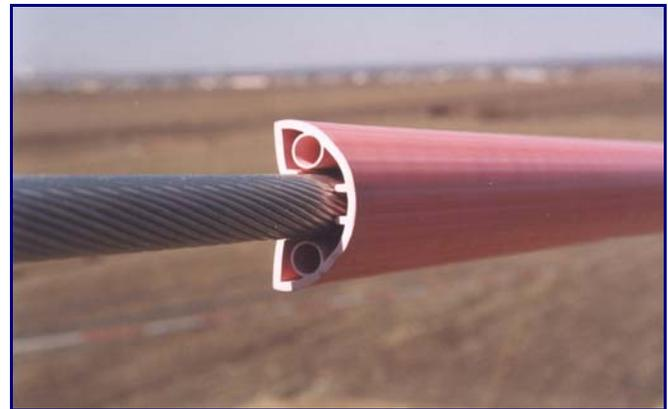
Fig. 7: D-section on conductor to produce galloping motions
