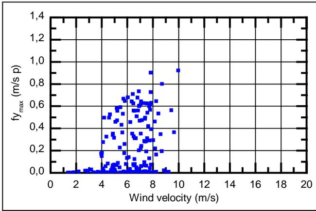
Fig. 14:  $f_{y_{max}}$  at 55% RTS for the 46 remaining days of the galloping test
