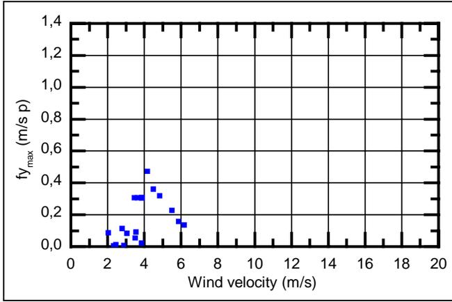
Fig. 13:  $f_{y_{max}}$  at 55% RTS after six days of the second galloping test
