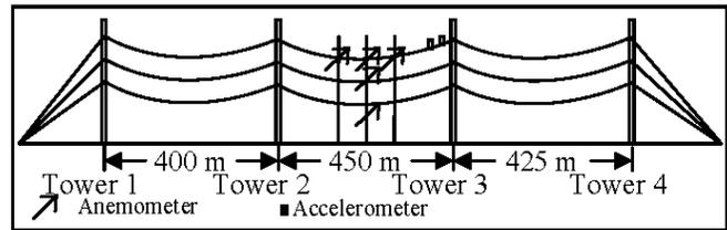
Fig. 5: Varennes test line layout for galloping tests
