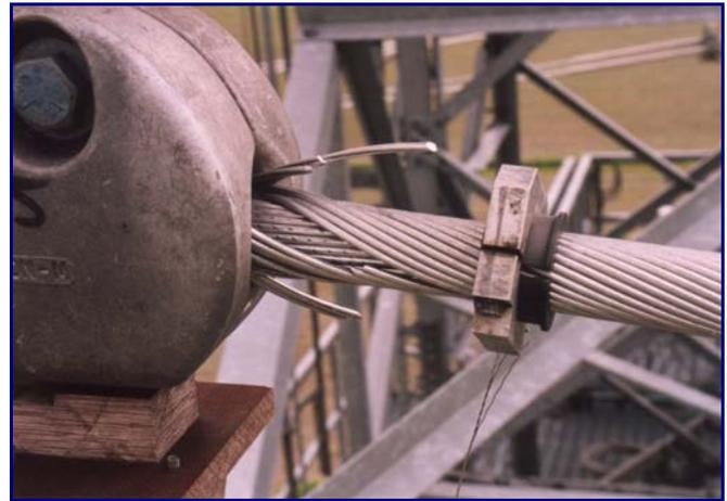
Fig. 11: Damaged conductor under the metal-to-metal clamp in the 450-m span after six day of the second galloping test
