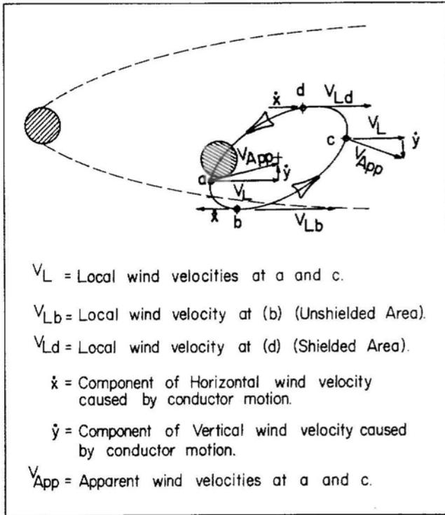
Fig. 3: Typical orbit of a circular cylinder in the wake of another cylinder [2]
