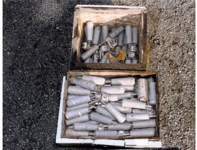
Fig. 2: Stockbridge dampers damaged during galloping tests at IREQ's test line
