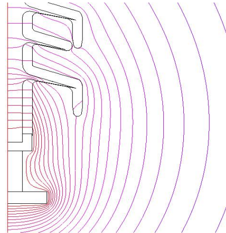
Fig.6 Potential contours around the composite insulator with 10mm icicles
