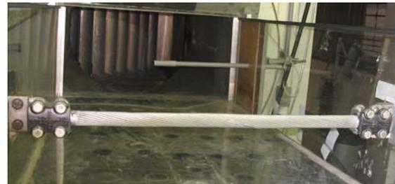
Fig. 3. The test section of the line conductor installed in the wind tunnel.
