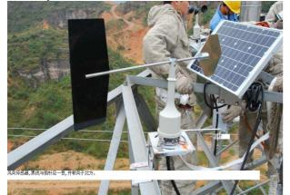
(g) wind direction sensor and solar bar
