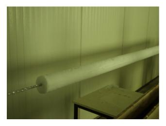
Fig.1. Snow sleeve on the suspended cable at the beginning of an experiment (the removed mold can be seen on the right side of the snow sleeve)
