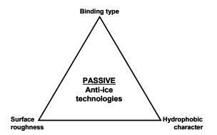
The Lotus effect is an example of surfaces that prevent wetting due to the combination of nano-scale and micro-scale surface structures and hydrophobic wax crystals. This leads to super-hydrophobic surfaces with water contact
