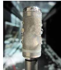
Fig.7 Ice accretion on the transducer
