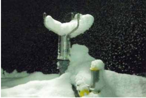
Fig.8 Snow accumulation on WS425
