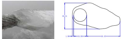
(b) conductor model: LGJ-185, temperature:  $-5\sim 0^{\circ}\text{C}$ , humidity: 97%, wind velocity: 3~9m/s, wind direction: horizontal axis and the wire into  $60^{\circ}\sim 90^{\circ}$ .
