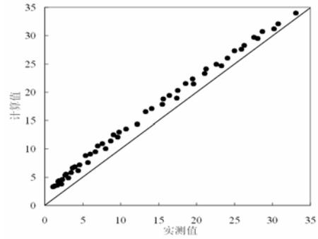
(a) Deviation between the calculated value and the ice thickness measured in field by equation (9) and (4)
