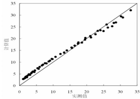
(b) Deviation between the calculated value and the ice thickness measured in field by equation (8) and (4)
