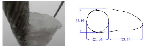
(c) conductor model: LGJ-240, temperature:  $-5\sim 0^{\circ}\text{C}$ , humidity: 97%, wind velocity: 3~9m/s, wind direction: horizontal axis and the wire into  $60^{\circ}\sim 90^{\circ}$ .
