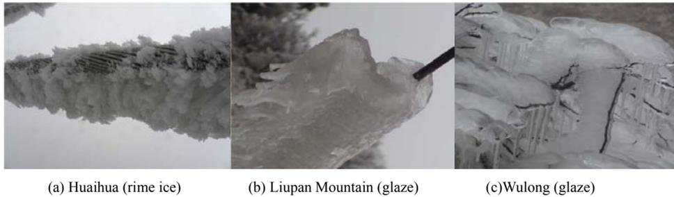
Figure 7. Icing shape observed in field
