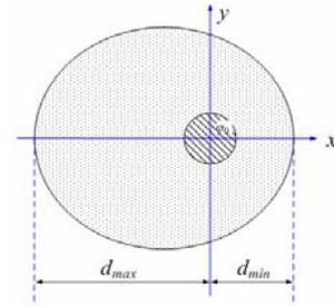
Figure 3. Elliptic icing conductor
