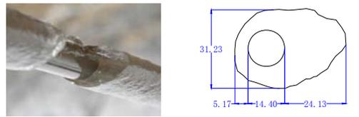
(a) conductor model: CTMH150, temperature:  $-3\sim 0^{\circ}\text{C}$ , humidity: 98%, wind velocity: 3~7m/s/wind direction: horizontal axis and the wire into  $60^{\circ}\sim 90^{\circ}$ .
