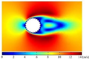
Figure 2. The airflow field around the conductor
