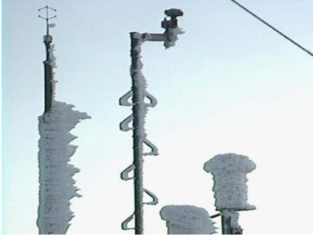
Figure 2. The ISO ice collector iced up at Ylläs (right). Ice mass on the 1 m long ISO collector at this time was 117 kg. i.e. Ice Class is R10. The non-cylindrical shape ("ice cap" on the top) is typical for ice accretions this large, but not for smaller ones.
