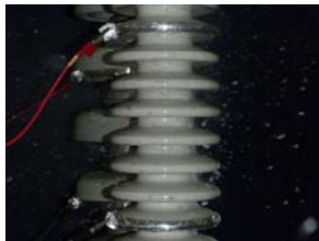
Figure 6. An example of snow flakes blown off the sheds by strong wind.
