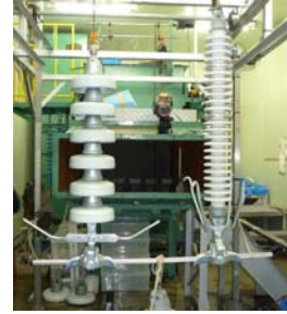
Figure 4. Set up of artificial snow accretion test.
