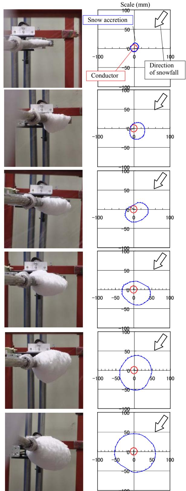
Figure 8. Comparison of the shape of snow accretion (L : Experimental results, R : Numerical computing results)
