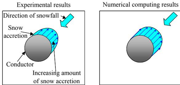
Figure 9. The shape of snow accretion in the early step
