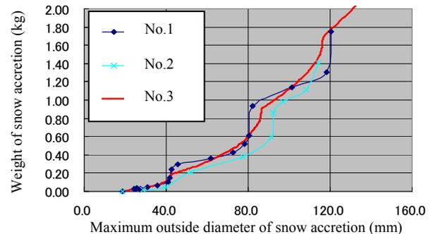
**Figure 1:** Comparison of the data (the weight : the maximum outside diameter of snow accretion)
