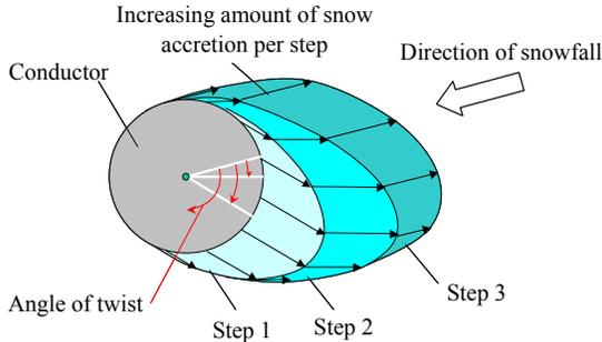
Figure 3. Growing process of snow accretion (detail)
