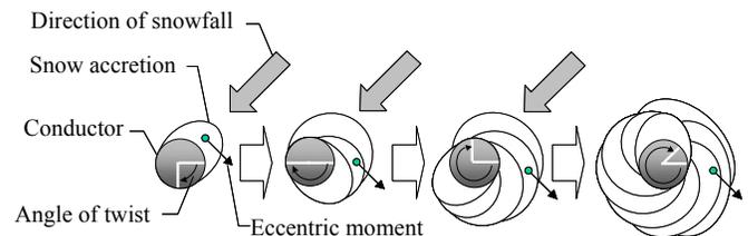
Figure 1. Growing process of snow accretion on a small outside diameter conductor having a long span (cross section)
