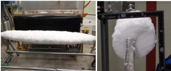
Figure 6. Snow accretion conditions at the end of the experiment (No.2)
