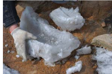
Figure 5. Icing shedding sample on grading ring of 667th
