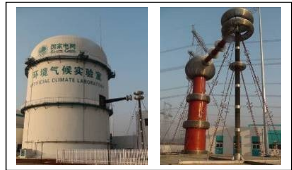
Figure 2. Hall of the climate laboratory and the experimental electrical source of power frequency
