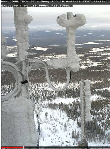
Figure 1. Ice Monitor (bottom) and Holooptics (top) ice measuring devices with some ice accretion on them.
