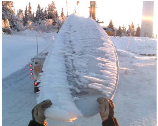
Figure 3: Ice collected on a wind turbine blade.
