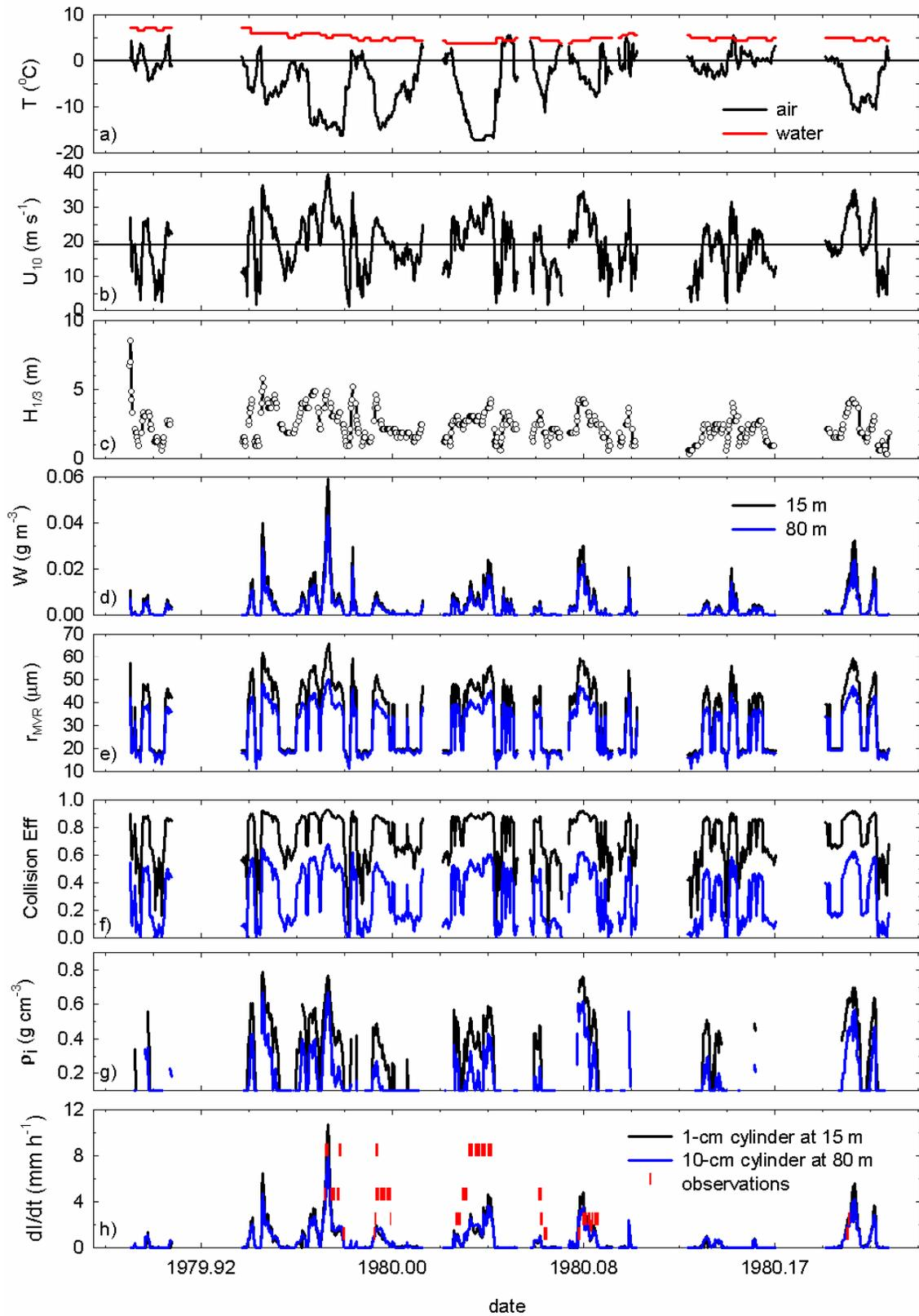
Figure 3. Ocean Bounty observations and simulations, winter of 1979-1980 a) air temperature, b) wind speed at 10 m, c) significant wave height, d) sea spray liquid water content, e) sea spray median volume drop radius, f) average collision efficiency, g) density of accreted ice, h) icing rate.
