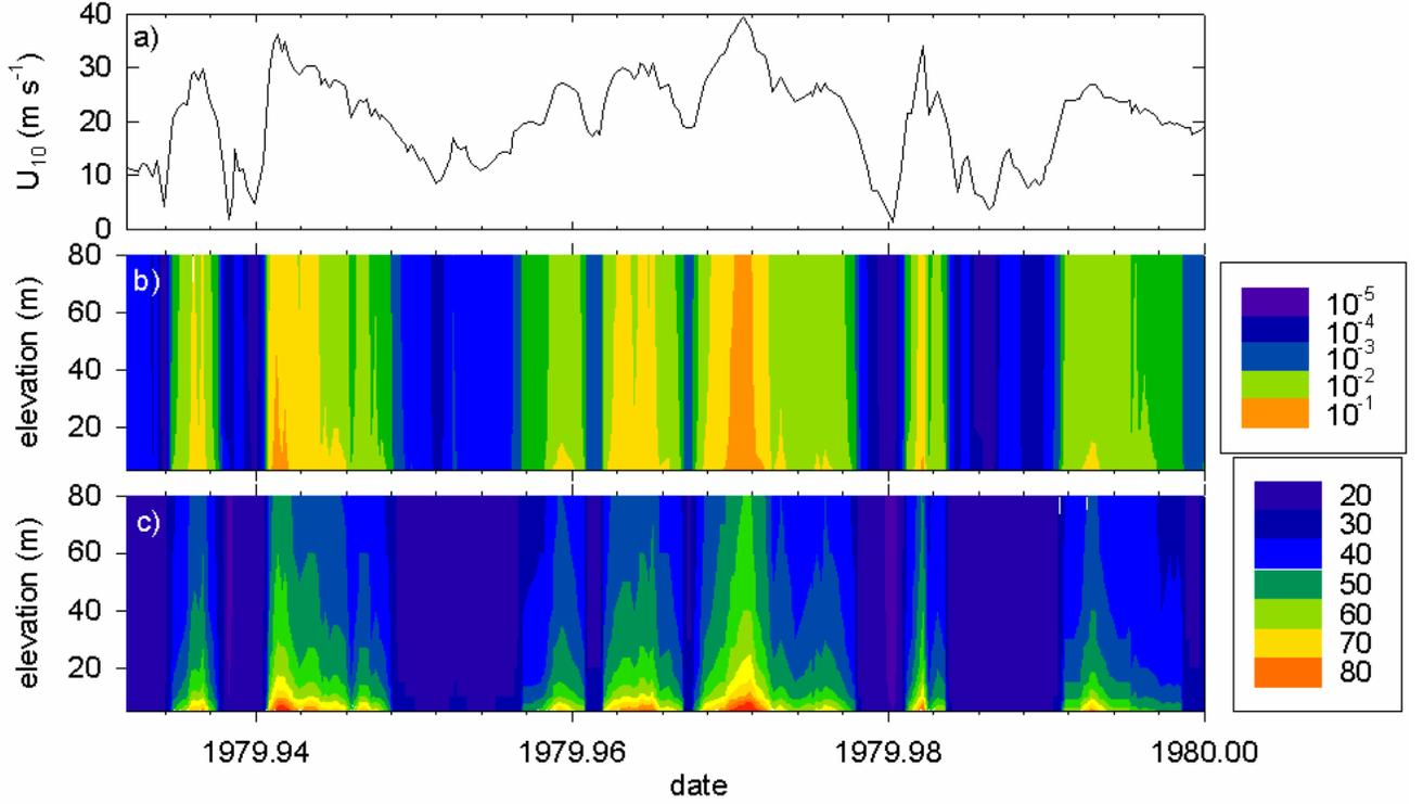
Figure 2. a) Wind speed at 10 m on the semisubmersible Ocean Bounty for the last 3 weeks and 3 days of 1979, b) simulated sea spray liquid water content, and (c) simulated median volume drop radius.
