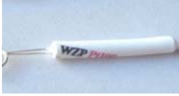
Figure.1 Pt100 platinum thermistor
