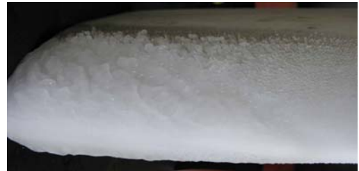
Fig.1 Icing test of airfoil surface in icing wind tunnel ( t=-5^\circ\text{C} , V=8\text{m/s} )
