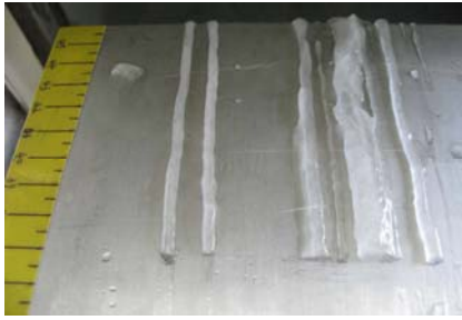
Fig.8 Runback icing test in icing tunnel
