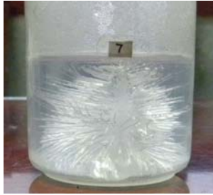
Figure 3 The freezing water in the monitor cup transition from liquid to solid phase completely
