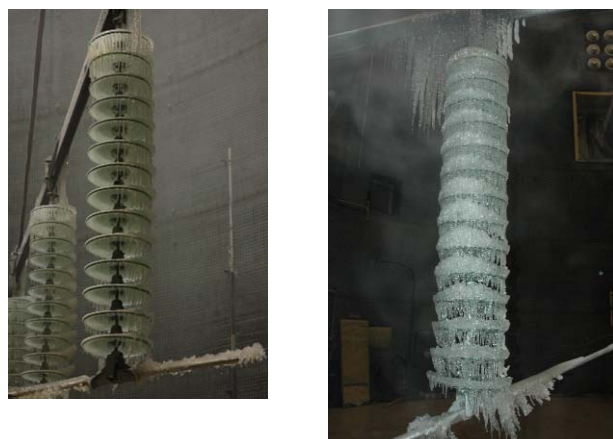
Figure 5. Development of ice accretion on insulators strings without MCS. Photos show examples after 5 h and 7 h of ice accretion.
