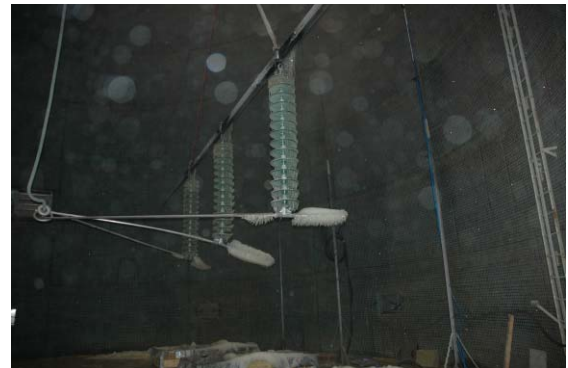
Figure 3. Set-up for ice accretion on insulator strings.
