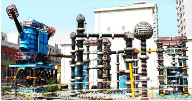
**Figure 2:** ±600 kV DC power supply.
