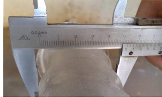
**Figure 5:** Thickness measurement of ice.
