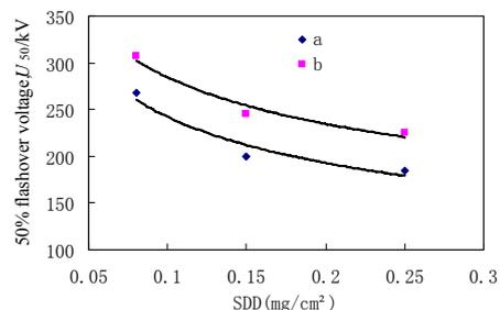
Fig. 5 the relationship between the 50% icing flashover voltage and  $SDD$
