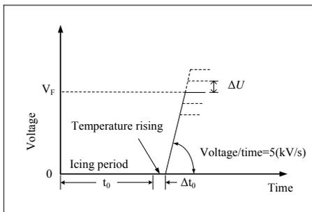
Fig. 2 The test method of 50% icing flashover voltage
