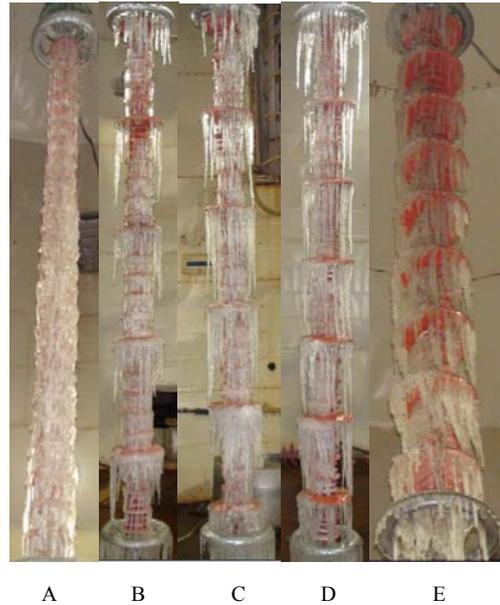
Fig. 3 Icing state of insulators of different shed profiles
