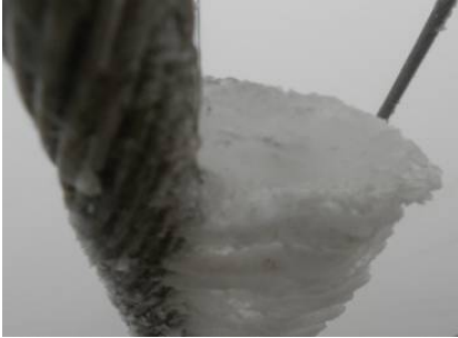
Figure 8. The shape of ice on sub-conductor of four bundled-conductor
