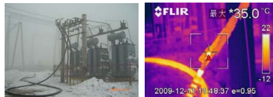
Figure 4: On-site De-icing Processes of Experimental Conductor
