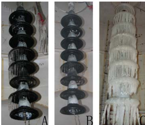
Figure 7. Result of ice accumulation test
