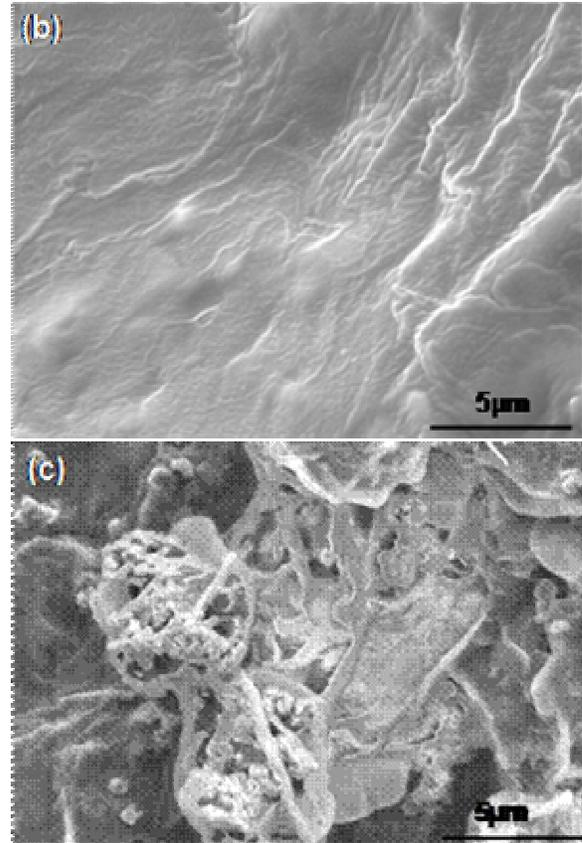
Figure 4. FESEM images of sample surfaces coated with different weight ratio of stearic acid. (a) 0; (b) 14 ;(c)43 wt.%
