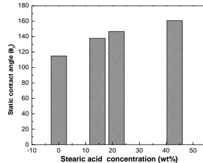
**Figure 1:** Evolution of water contact angle as a function of stearic acid concentration (wt. %)
