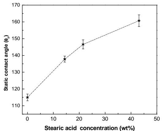
Figure 2. Evolution of water contact angle as a function of stearic acid concentration (wt. %)
