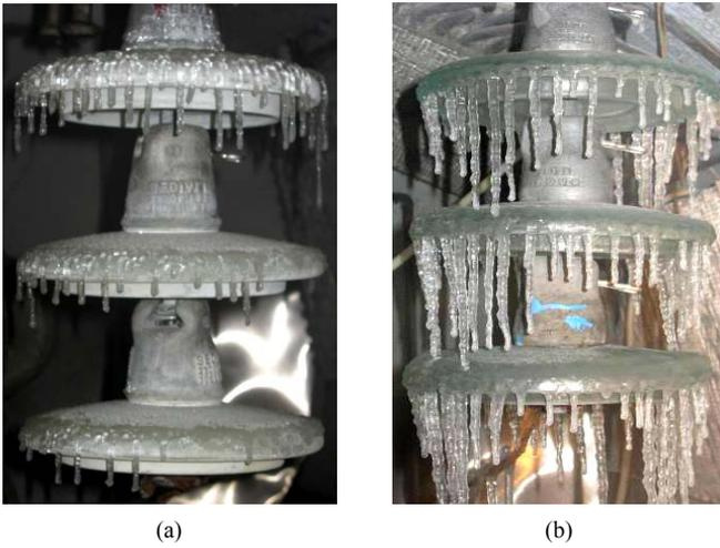
Figure 4 Photographs of accumulated ice on different types of insulator strings under icing condition
