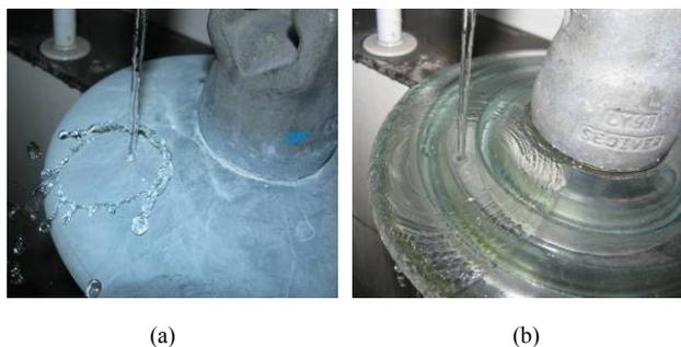
**Figure 2** Water flowing on surface of different types of insulator
