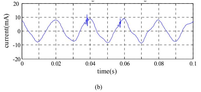
Figure 5 Leakage current waveforms of different types of insulator strings under icing condition
