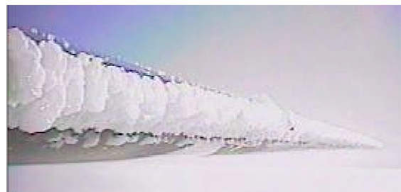
Figure 1. Ice accretion on wing during natural flight tests
