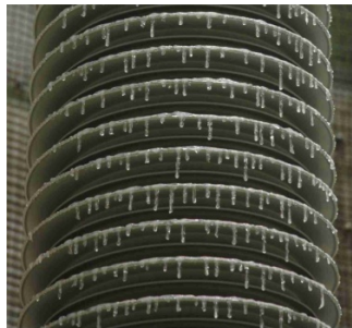
Figure 6. Close-up of the insulators with ice before the test with salinity 30 \text{ kg/m}^3 . Porcelain insulators are shown at the top and silicone rubber insulators is shown at the bottom.
