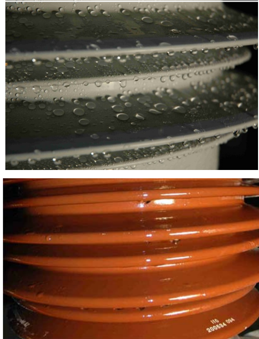
Figure 4. Hydrophobicity evaluation of the insulators after the three salt fog tests (10-20-30 kg/m 3 ) at low temperature: silicone rubber insulator at the top; porcelain insulator at the bottom.
