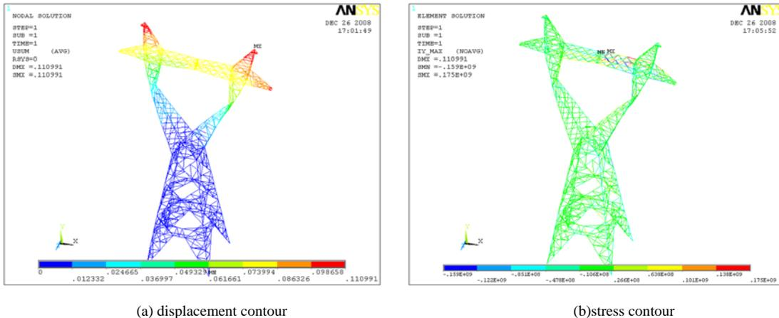
Figure.1 Tower Displacement and Stress Contour of Border Signal Phase Conductor De-icing.
