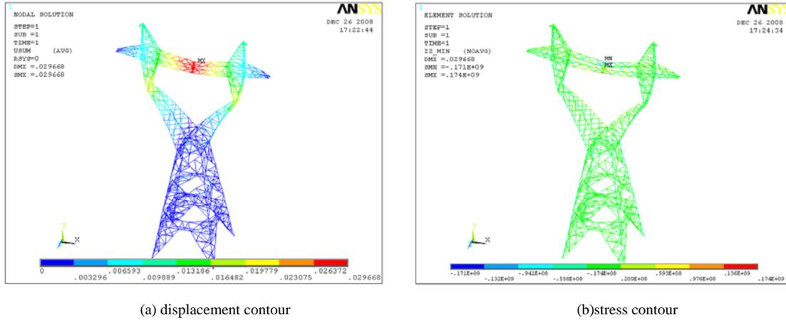
Figure.4 Tower Displacement and Stress Contour of Both Border Phases Conductors De-icing.
