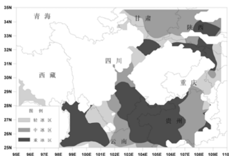
Fig 4. Spatial distribution of mean icing intensity (risk) in recent 50 years in Southwest China
